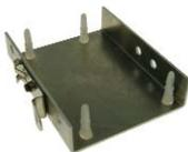
DIN Rail mounting bracket enables any module which can be mounted to a M520 ancillary cover to be DIN rail mounted using this bracket. Clip-on PCB mounting pillars are included. Will fit standard 35mm DIN Rail bracket.
