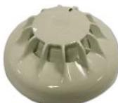
The CO fire detector is a unique general purpose fire detector which provides very early warning of slow smouldering fires. Ideal for sleeping risks the CO fire detector is also well suited to many applications where heat detection is insufficient but smoke detection causes false alarms. As CO travels more freely than smoke the position of CO fire detectors is more flexible.
