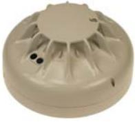
Complementing the range is the heat sensor which can operate in fixed temperature and rate-of-rise modes with a number of approved sensitivities. It is most often used in areas where high levels of dust are present or where the environment precludes the use of smoke detectors.
