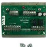
The VIO800 MX Vesda Interface will enable all versions of the popular LaserPLUS Detectors and 7 relay versions of the Laser SCANNER Detectors to be interfaced directly to the MXDigital detection loops. 3 configurable inputs and 1 output signal are available from the interface enabling it to integrate fully with the Vesda detector.
