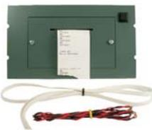
The PRN800 Printer Kit is designed for use with the designer range of MX Controllers (MX4000 and T2000). It is fitted to the front cover of the MX battery housing and is powered from the PSB 800 power supply via an FB800 fuseboard in the MX Controller housing.
