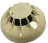
These detectors are capable of detecting the visible smoke produced by materials which smoulder or burn slowly, i.e. soft furnishings, plastic foam etc.; or 'smoke' produced by overheated but unburnt PVC. These detectors are particularly suitable for general applications and areas where cable overheating may occur e.g. electrical services areas. The novel design of the asymmetrical sampling chamber and signal processing techniques stop unwanted alarms caused by very small insects. i.e.
