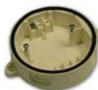
Where the detectors are mounted in humid and environmentally challenging situations such as marine or offshore installations, the 4B-DHM deck head mount provides a sealed waterproof mounting which protects the electrical connections in the base. Can be screwed, bolted / welded to the deckhead. Supplied with 1 terminal. If more are required,
