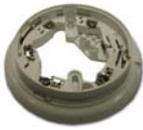
The 5BD Continuity Base is a standard 5 inch base fitted with a continuity diode, for use with all Series 600 detectors. The base is designed to ensure that conventional systems meet the requirements of BS5839 Pt:1 for callpoints placed after detectors.
