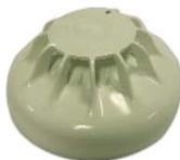
These detectors use two networked thermistors in a bridge configuration to provide a fast response, that depends both on absolute temperature and notes the change of temperature. The rate of rise/fixed temperature heat detectors can be used in areas where smoke sensors are unsuitable due to environmental conditions (smoke, dust etc.). Such areas include kitchens, locker rooms, canteens, garages, loading bays etc.
