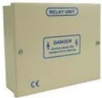
RU1-24, this is a metal boxed auxiliary relay with 5 A Mains rated double pole contacts with a 24 VDC 25mA coil. This compact relay is suitable for interfacing a fire alarm controller to low current mains powered devices or contactors
