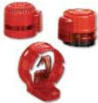
This low power LED beacon is designed to be retrofitted to existing Banshee electronic sounders. Easy and fast installation typically 3 min. Low power 6mA max at 24Vdc. High Output LEDs.
