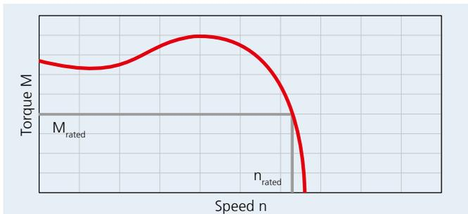
Typical torque characteristic curve for a squirrel cage motor
