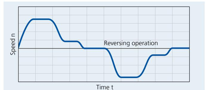
ZBA/ZNA motors tend to be used for applications involving reversing duty and creep positioning speeds
