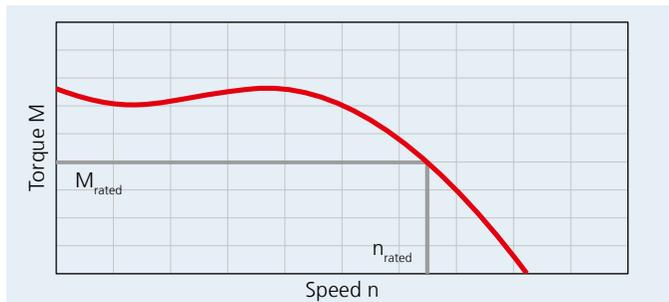
Constant smooth-start characteristics with no excessive starting and breakdown torque
