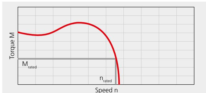
High starting torque for dynamic acceleration
