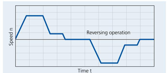
ZBF and KBF motors tend to be used for applications involving reversing duty with creep-positioning speeds.
