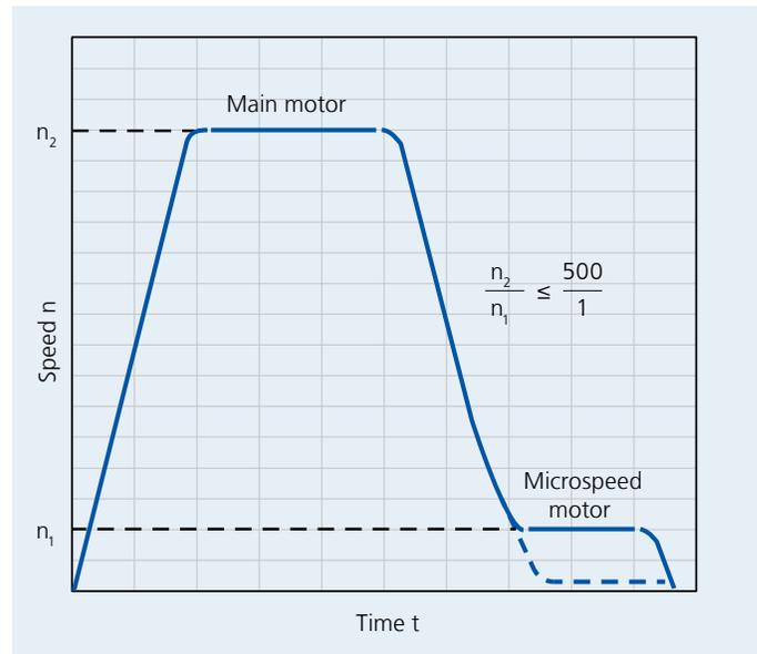
By selecting the right combination of motor and gearbox, the speed ratio can be set within a broad range
