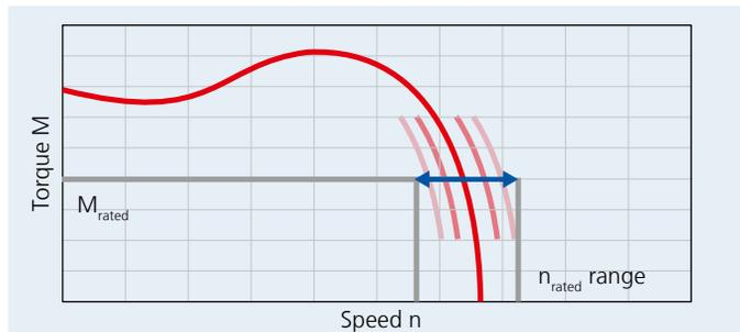
When using an inverter, it is possible to adjust the characteristic curve, which is optimized for travel applications
