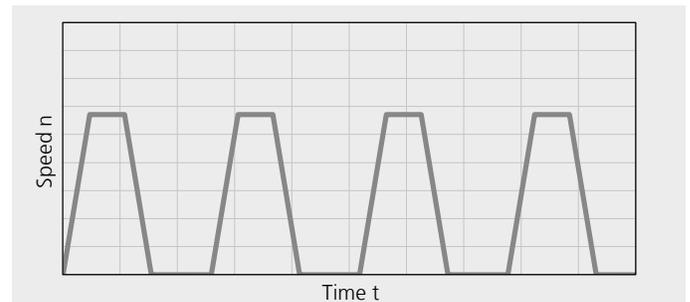
KBA motors are suitable for extremely high start-stop frequencies
