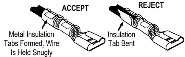
1. Be sure that the insulation barrel tabs are not bent.
