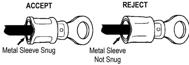
1. On closed barrel terminals that have a secondary metal sleeve (AviKrimp™), the metal sleeve should be formed snugly around the wire.
