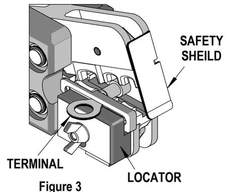
4. If using a locator, lift the locator and insert the terminal with the wire in the proper nest with the barrel up and against the locator bar. Release the locator blade to hold the terminal in position. See Figure 3. Locator may be raised or lowered so terminal sits flat and straight in tool. The locator must be removed to run splices.
