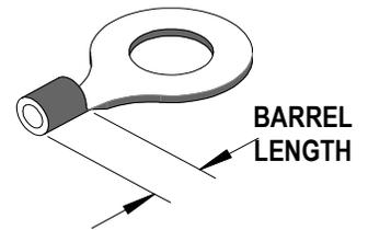
The purpose of the longer barrel is simply to give the user a bigger target area to crimp. These barrel lengths are not so important if you use a terminal with the molded step construction on the insulation, or if a precision ratchet tool with terminal locator is used. OEM tooling is usually designed for only short barrel terminals.
