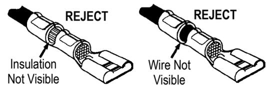
4. If there is no insulation support crimp, be sure that the length of the wire visible behind the conductor crimp is not greater than the diameter of the insulation. If the length of the wire visible exceeds the diameter of the insulation, the terminal could cause a short circuit.
