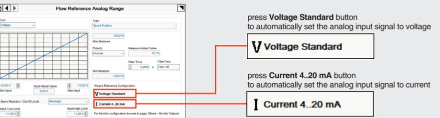
**REMARK:** **Voltage Standard** or **Current 4..20 mA** buttons do not act on Monitor output signal configuration!
