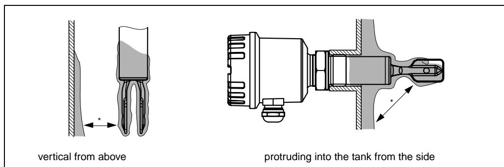
**Mounting positions with low viscosity (up to 2000 mm<sup>2</sup>/s):**
