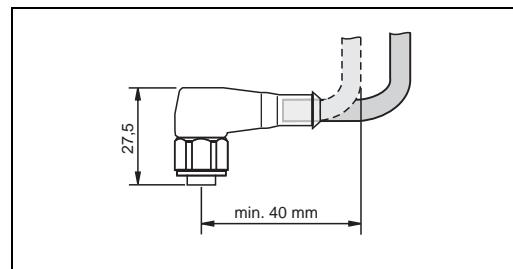
M12 x 1 connector without LEDs
