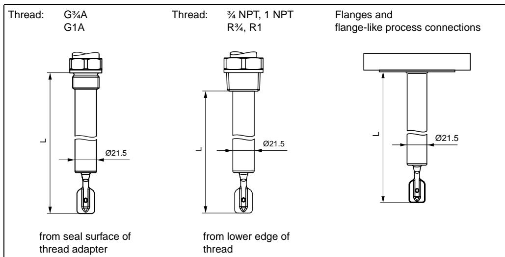
Extension tube: any length L 148 mm ... 3000 mm (6 in ... 115 in), special version on request up to 6000 mm (20 ft)
