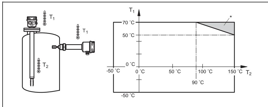
\* additional temperature range for devices with a temperature spacer or pressure-tight bushing
