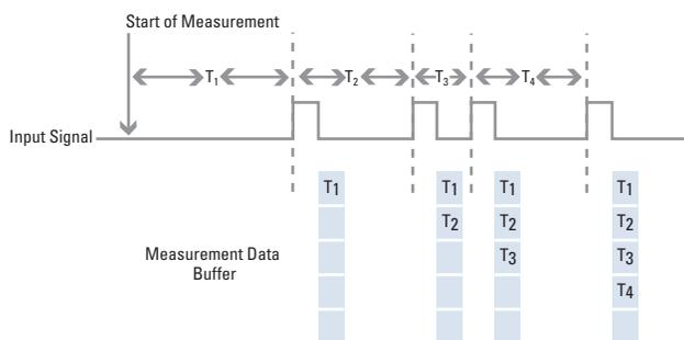
Figure 1. Buffered Period Measurement with Counter/Timers
