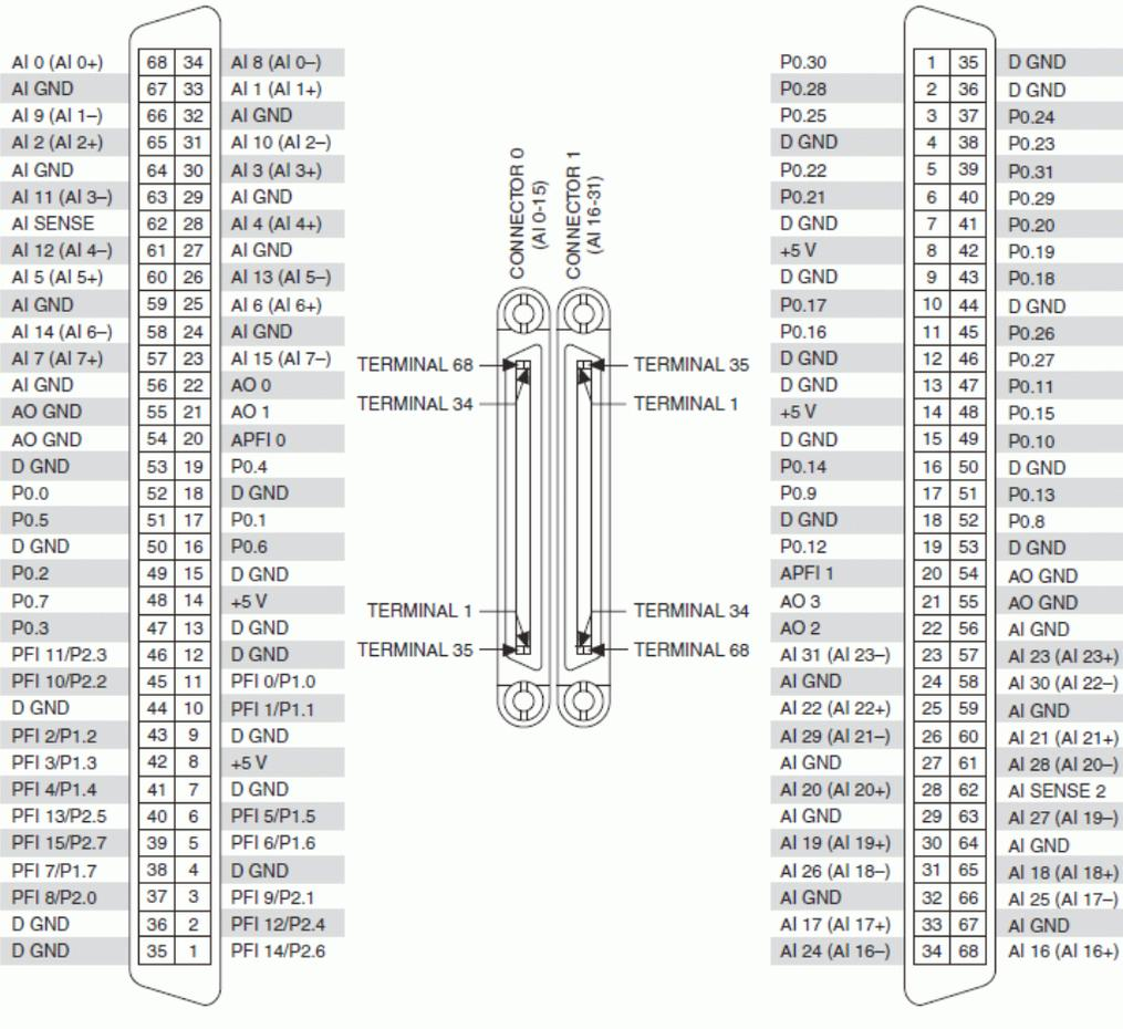
NI PCIe/PXle-6363 Pinout
