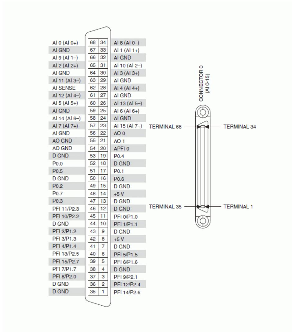
NI PCIe/PXIe-6361 Pinout
