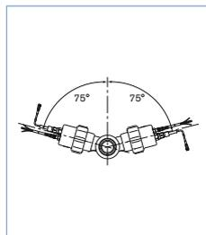
The device has to be installed with a maximum angle of 75 degrees against the vertical onto an horizontal pipe. Select and install the required fitting onto the pipe, according to specific requirements of the device and fitting material (temperature and pressure). After having connected the device to the Type 8619 (pH/ORP) multiCELL transmitter/controller and having calibrated the unit, cautiously install the complete pH/ORP meter on the fitting.
