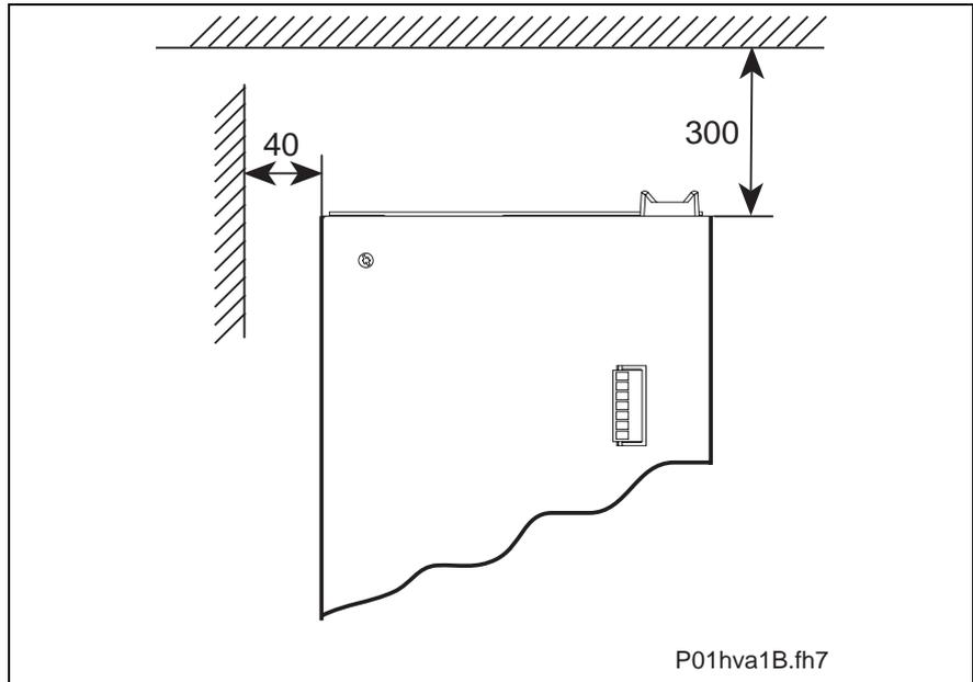
Fig. 7-11: Safety distance of the bleeder resistor
