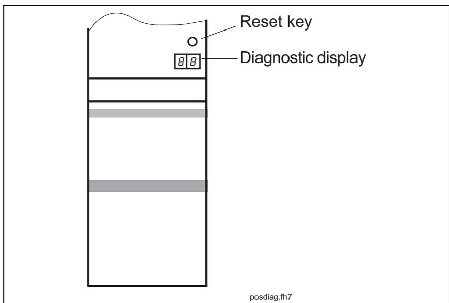
Fig. 11-1: Position of diagnostic display and reset key
