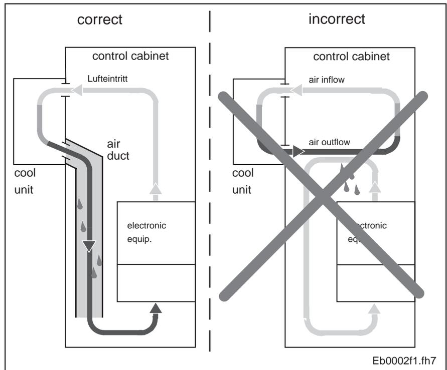
Fig. 7-7: Cooling unit arrangement on the front of the control cabinet
