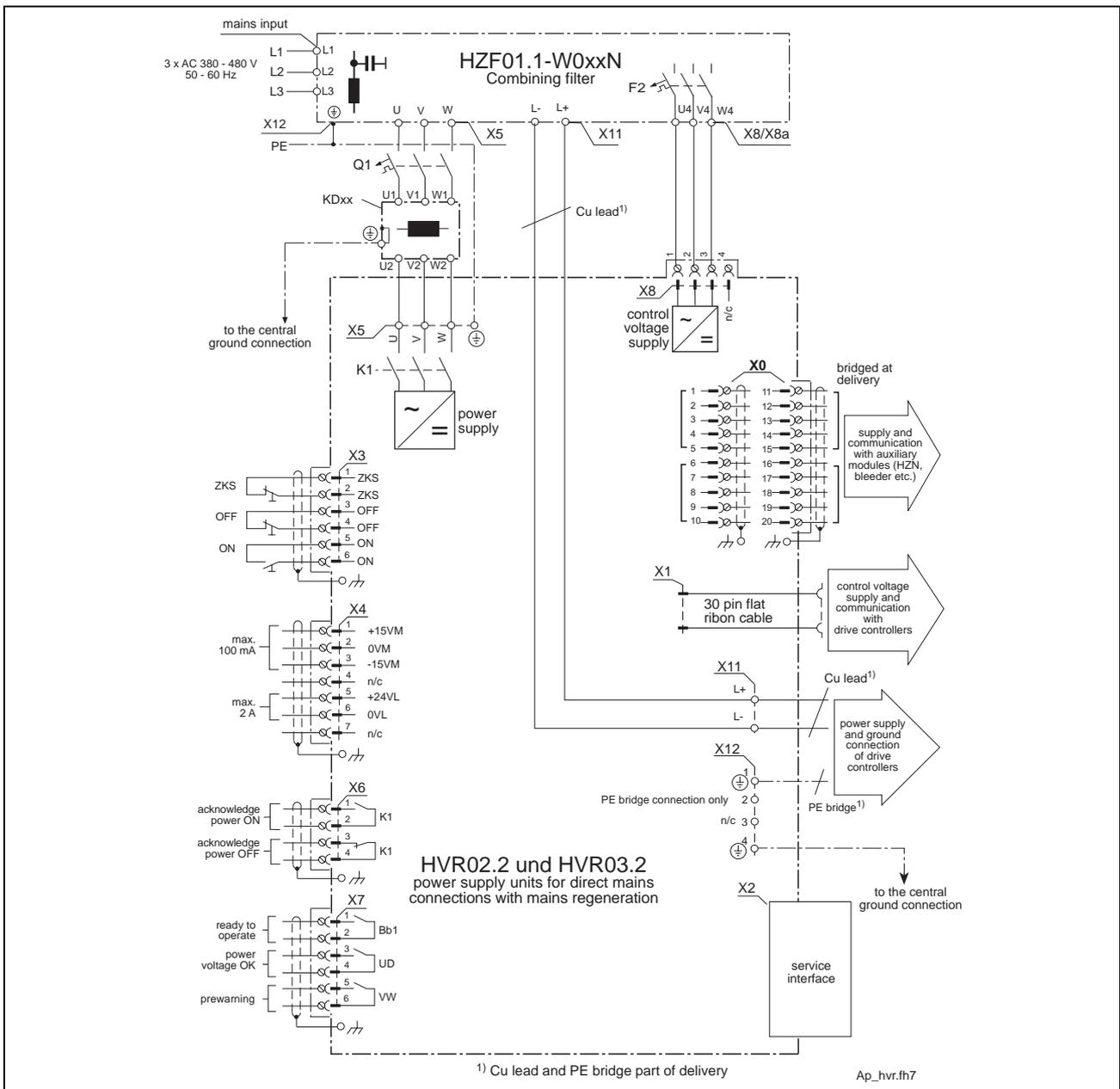
Fig. 8-5: Terminal diagram for HVR02.2 and HVR03.2
