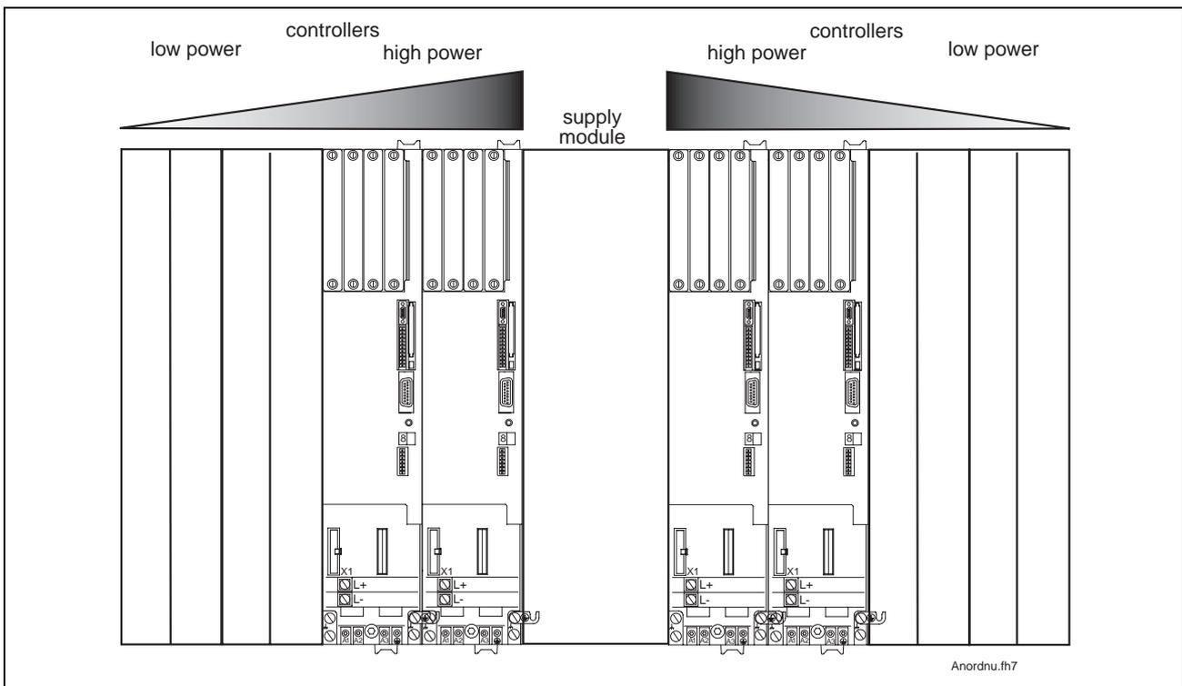
Fig. 7-10: Recommended unit arrangement within the control cabinet
