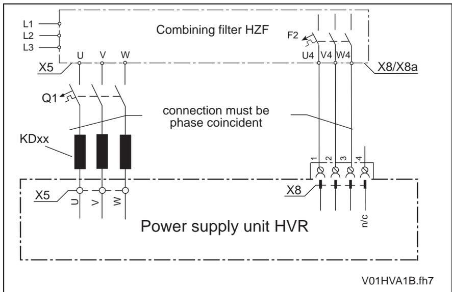
Fig. 8-11: HVR control voltage
