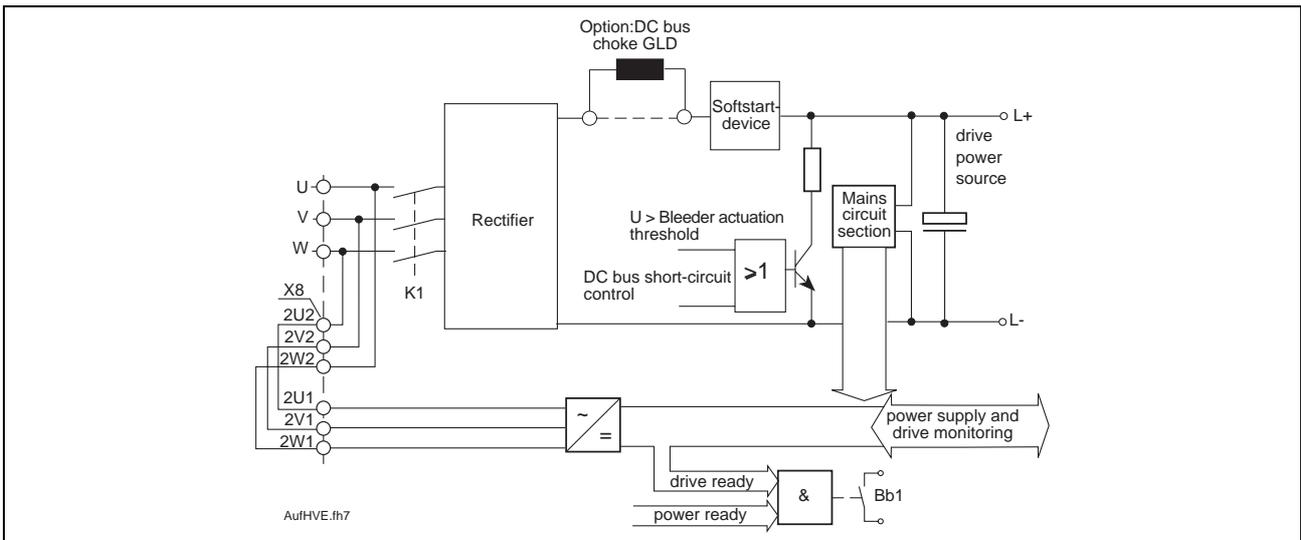
Fig. 1-2: Structure of the HVE power supply unit
