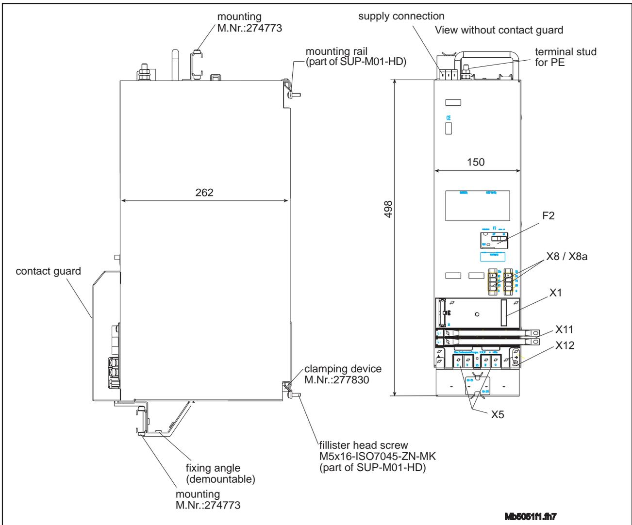
Fig. 7-20: Dimension drawing HZF01.1-W010N
