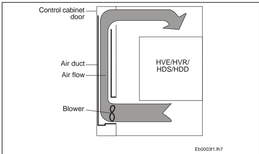
Fig. 7-9: Control cabinet with air circulation system
