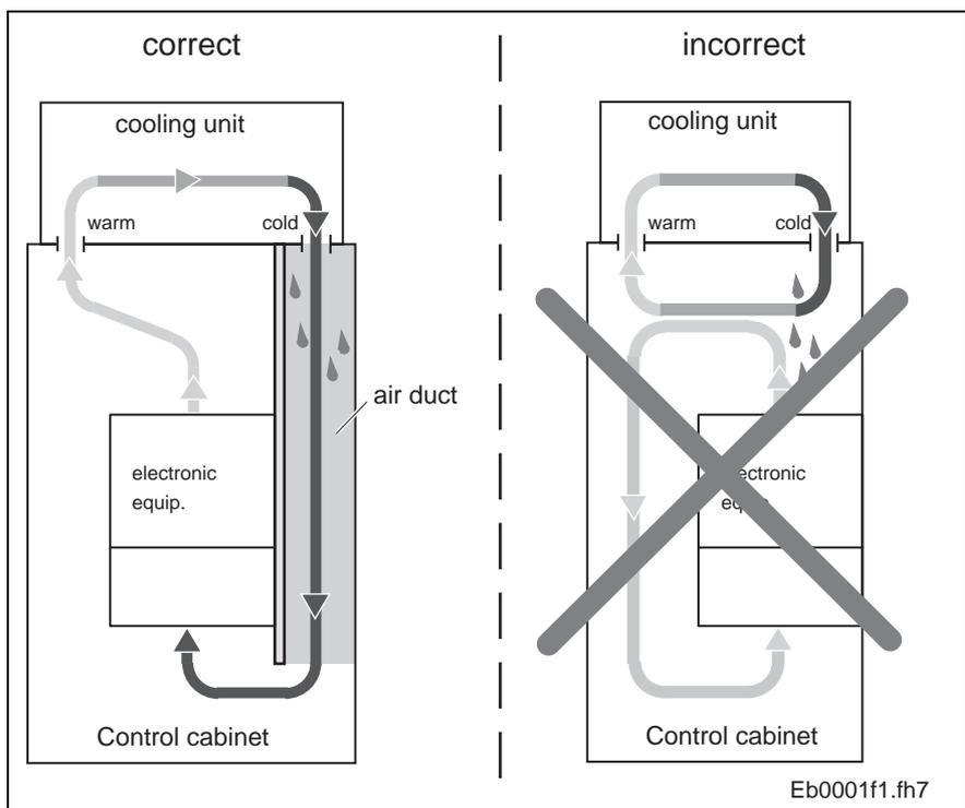
Fig. 7-6: Cooling unit arrangement on the control cabinet
