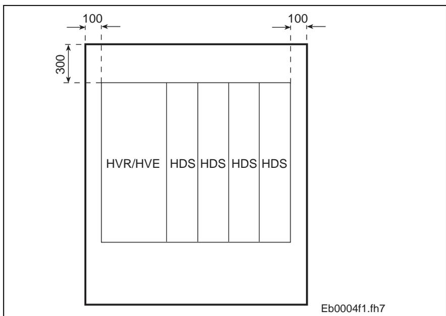
Fig. 7-8: Control cabinet (uncooled, unventilated) with drive package
