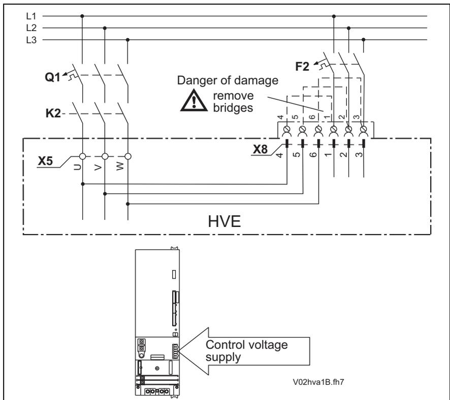
Fig. 8-9: Separate control voltage sources for the HVE
