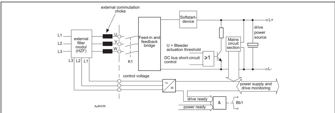
Fig. 1-3: Structure of the HVR power supply unit
