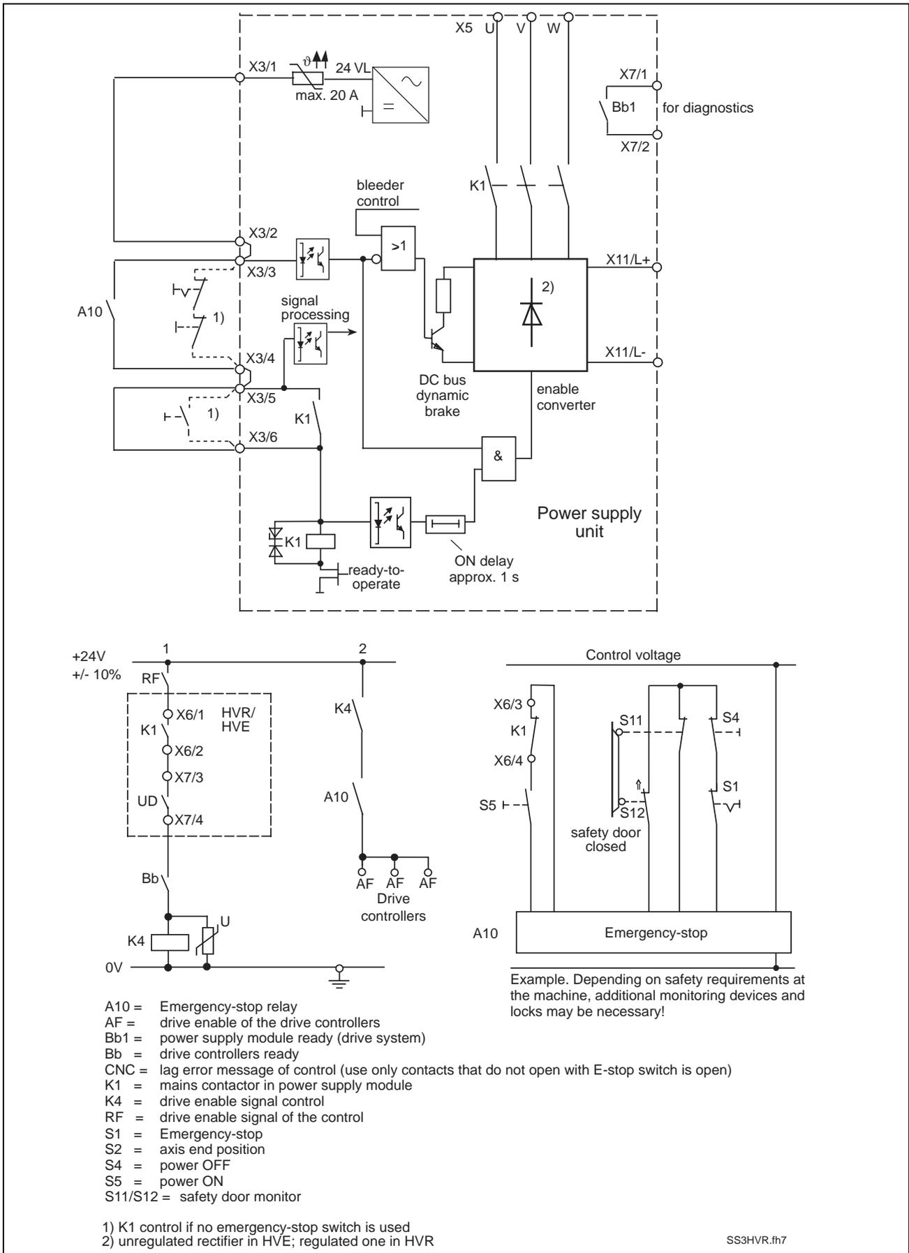
Fig. 9-2: Control of the power supply unit without DC bus dynamic brake
