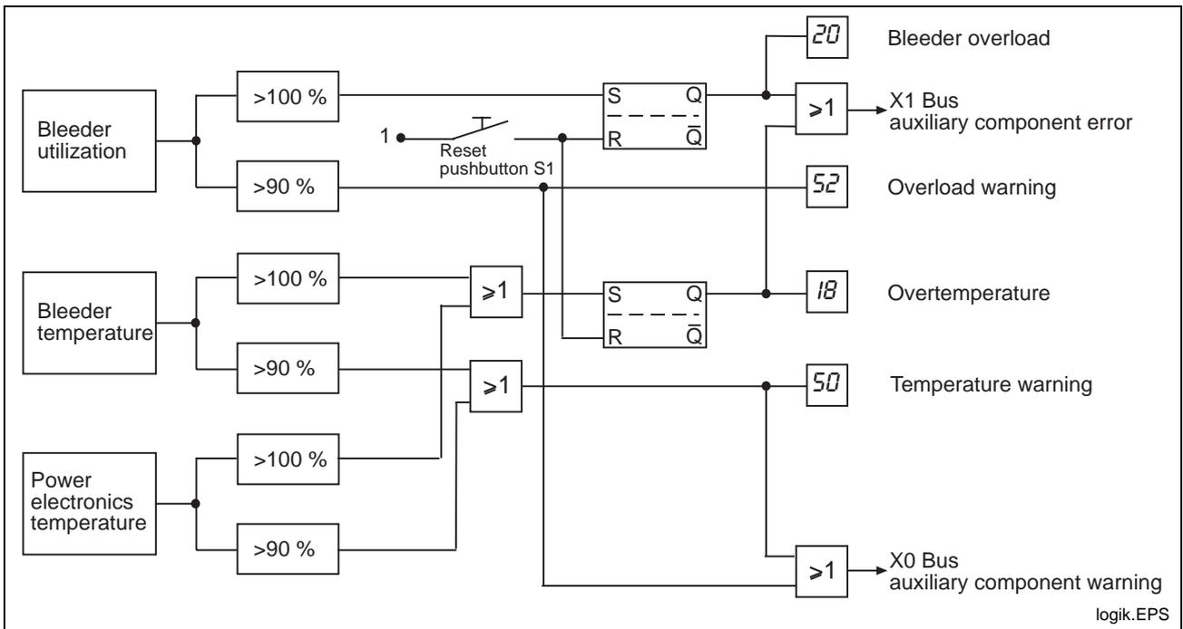
Fig. 6-7: Monitoring and diagnostic logic HZB02.2-W002N
