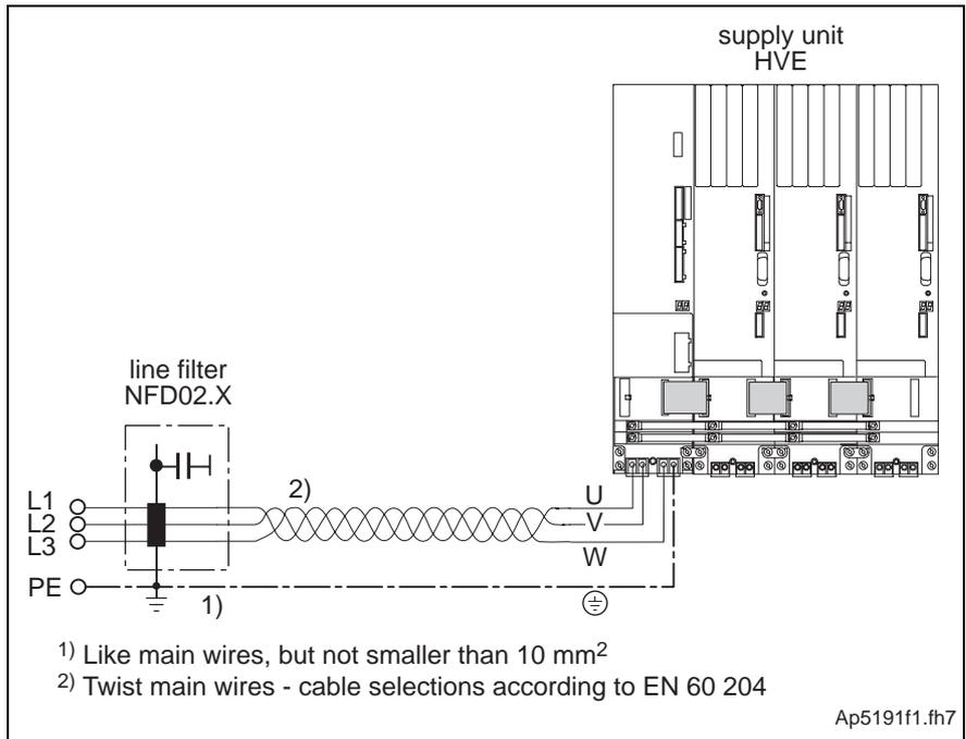
Fig. 8-7: Direct mains connection via line filter NFD02.x
