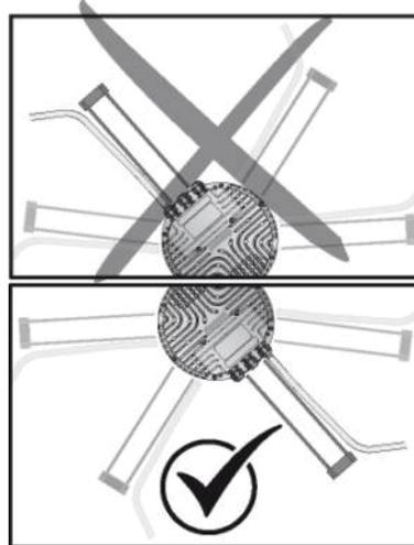
Fig. 4: Cable routing for fans installed upright.
