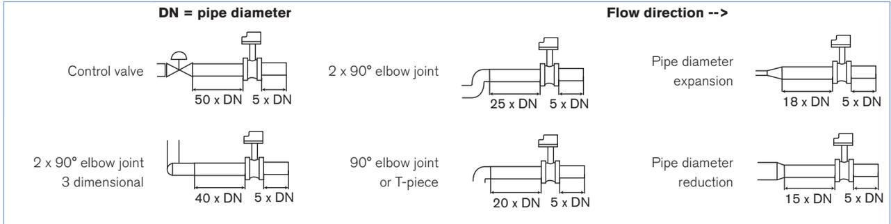
The device can be installed into either horizontal or vertical pipes. Mount the 8035 in these correct ways to obtain an accurate flow measurement.
