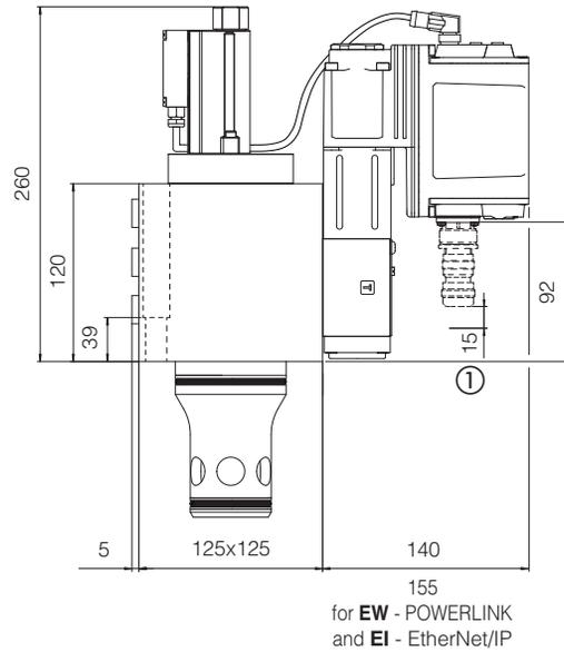
① Space to remove the 7 or 12 pin main connector. For main and communication connectors see section 11, 12
