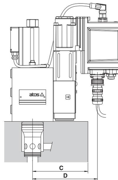
**C** = Max manifold dimension to avoid interference with the main connector, see below table
