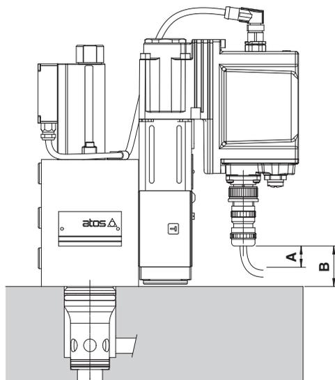
**A** = 15 mm space to remove the 7 or 12 pin main connectors
