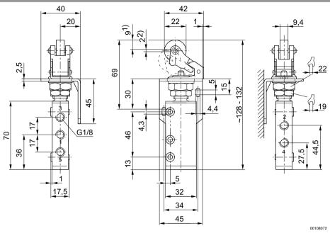
1) actuating stroke 2) overstroke Can be adjusted by 90  $^\circ,$  thereby providing 4 different angles of approach.
