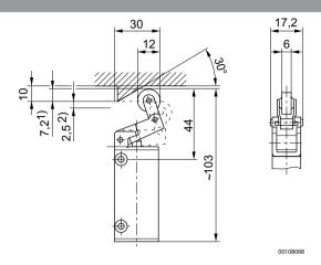
1) Actuating stroke 2) overstroke connection via 2 through-holes in housing
