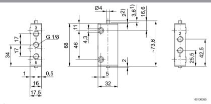
1) actuating stroke 2) overstroke connection via 2 through-holes in housing. If the plunger is displaced all the way to the housing cover, the actuating stroke changes from 3.6 to 5.6 mm.
