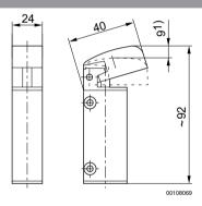
1) actuating stroke Mounting via 2 through-holes in housing
