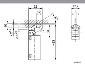
1) Actuating stroke 2) overstroke connection via 2 through-holes in housing
