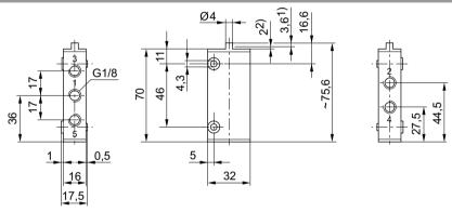
Actuating stroke 2) overstroke connection via 2 through-holes in housing Dimensions of basic valve apply to all types of actuation.
