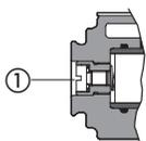
① = Screw for air bleeding: at the first valve commissioning the air eventually trapped inside the solenoid must be bled-off through the screw ①
