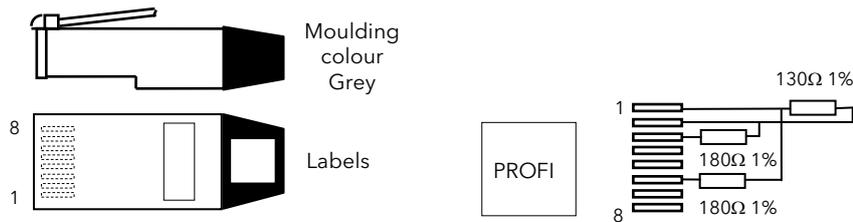
Figure 2-12: The Profibus RJ45 Terminator
