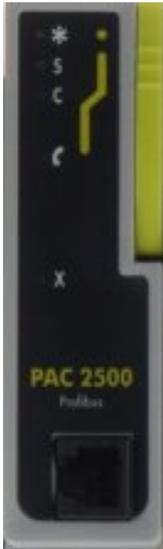
The Input / Output Controller module (IOC) is the central processing unit of the 2500 system.
