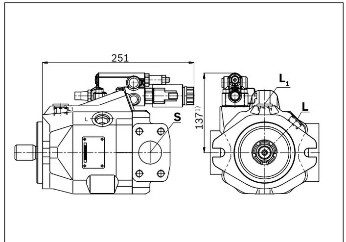
1) ER7.: 172 mm if using an intermediate plate pressure controller
