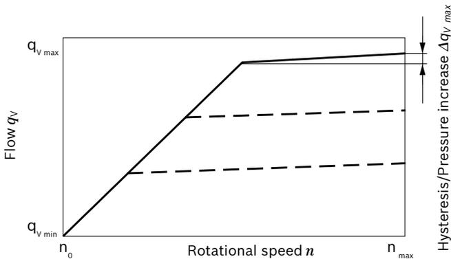
Characteristic curves valid for  $n_1 = 1500$  rpm and  $t_{fluid} = 50$  °C.
