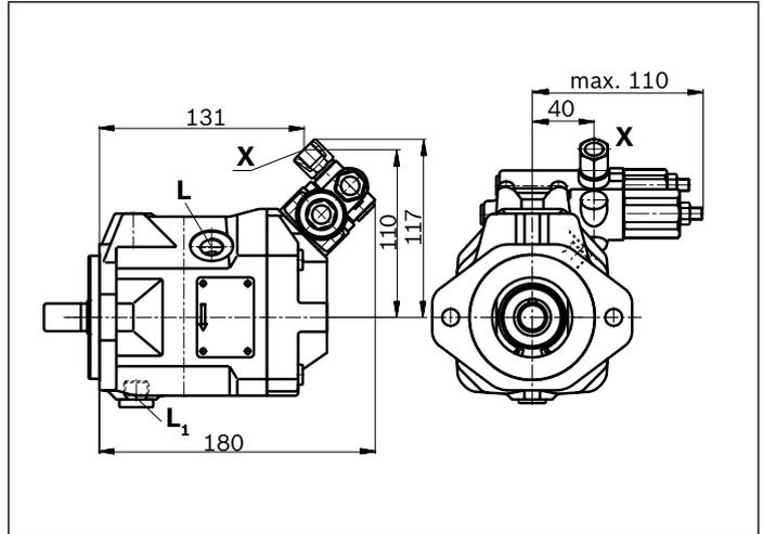
▼ **DRG – Pressure control, remotely operated (SAE)**<sup>1)</sup>
