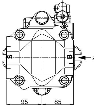
1) Dimensions of working ports turned through 180° for counter-clockwise rotation
