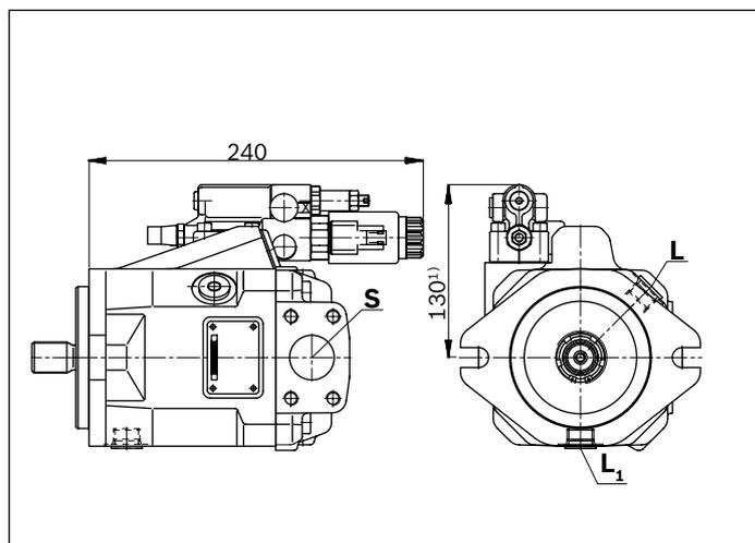
1) ER7.: 159 mm if using an intermediate plate pressure controller
