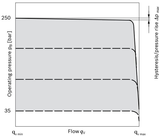
Characteristic curve valid for  $n_1 = 1500$  rpm and  $t_{\text{fluid}} = 50$  °C.
