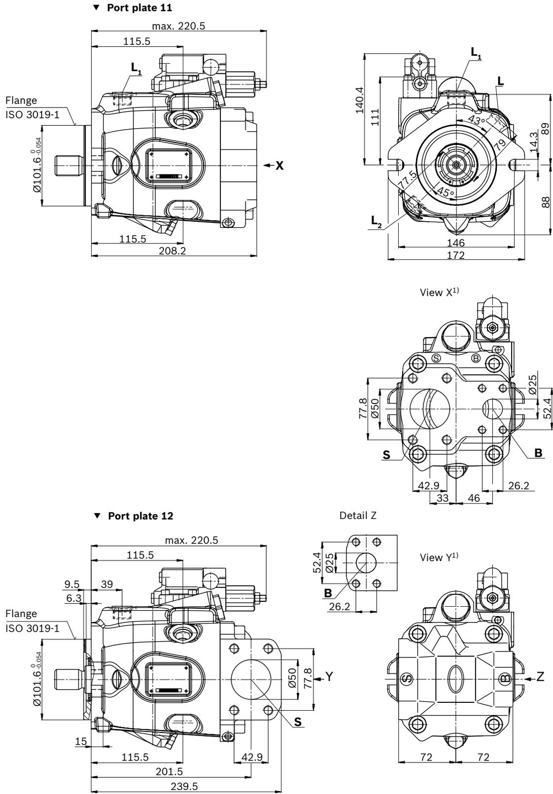
1) Dimensions of working ports turned through 180° for counter-clockwise rotation
