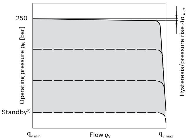
Characteristic curve valid for  $n_1 = 1500$  rpm and  $t_{\text{fluid}} = 50$  °C.
