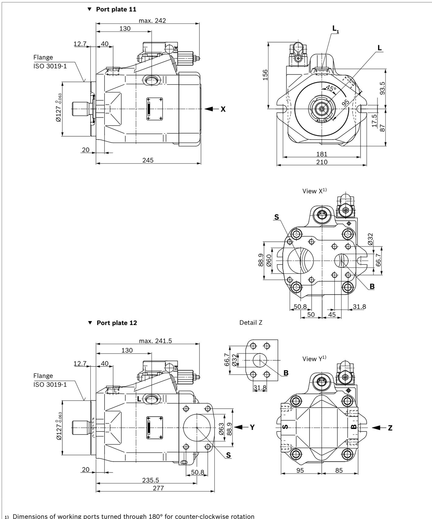
1) Dimensions of working ports turned through 180° for counter-clockwise rotation
