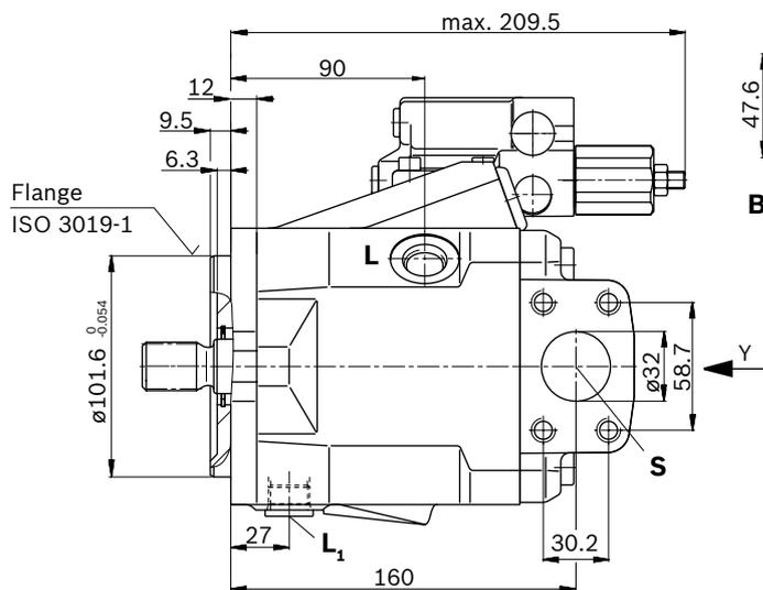
1) Dimensions of working ports turned through 180° for counter-clockwise rotation
