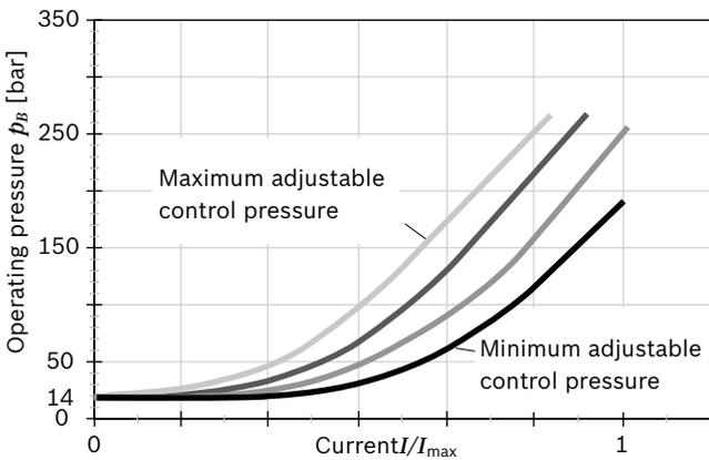
► Hysteresis static current-pressure characteristic curve < 3 bar.
