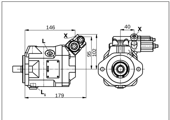
1) Valve mounting for clockwise or counter-clockwise rotation see page 11 and 12
