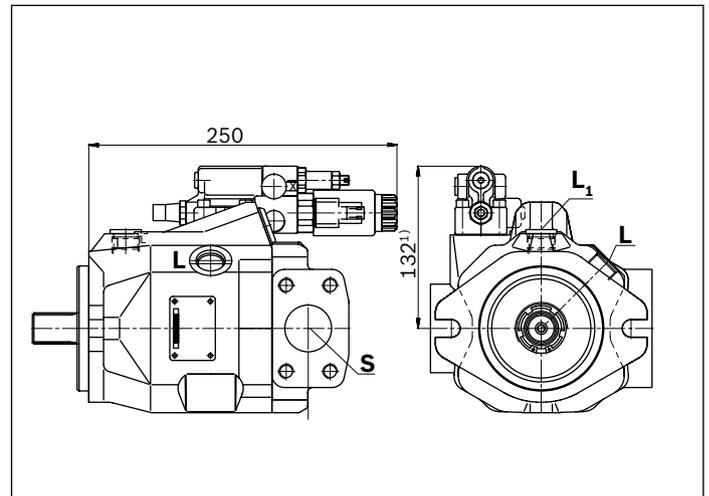
1) ER7.: 167 mm if using an intermediate plate pressure controller
