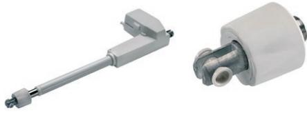
The purpose of the EL (Emergency Lowering) is in case of a powerfailure, to be able to mechanically lower a patient by turning the EL part in the clockwise direction until the actuator is fully lowered.
