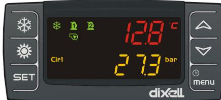
**Upper digits (red color):** configurable by parameter CF36 (PB1, PB2, PB4, Set-point (parameter value)\*, working set-point (real set-point modified from dinamic set-point, Energy saving or function for units without water storage tank), Hysteresis, Machine status \*\*)
