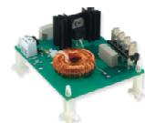
**CW15-KIT e CWC15-KIT:** Ichill wiring kit for 5 realsys model and 4 relays + 1 triac model
