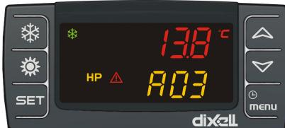
When the instrument detects an alarm, the lower display shows the alarm code alternated to probe value. The alarm icon ( $\Delta$ ) is on flashing.
