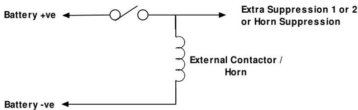
Figure 5: MillipaK Standard HP Light Wiring
