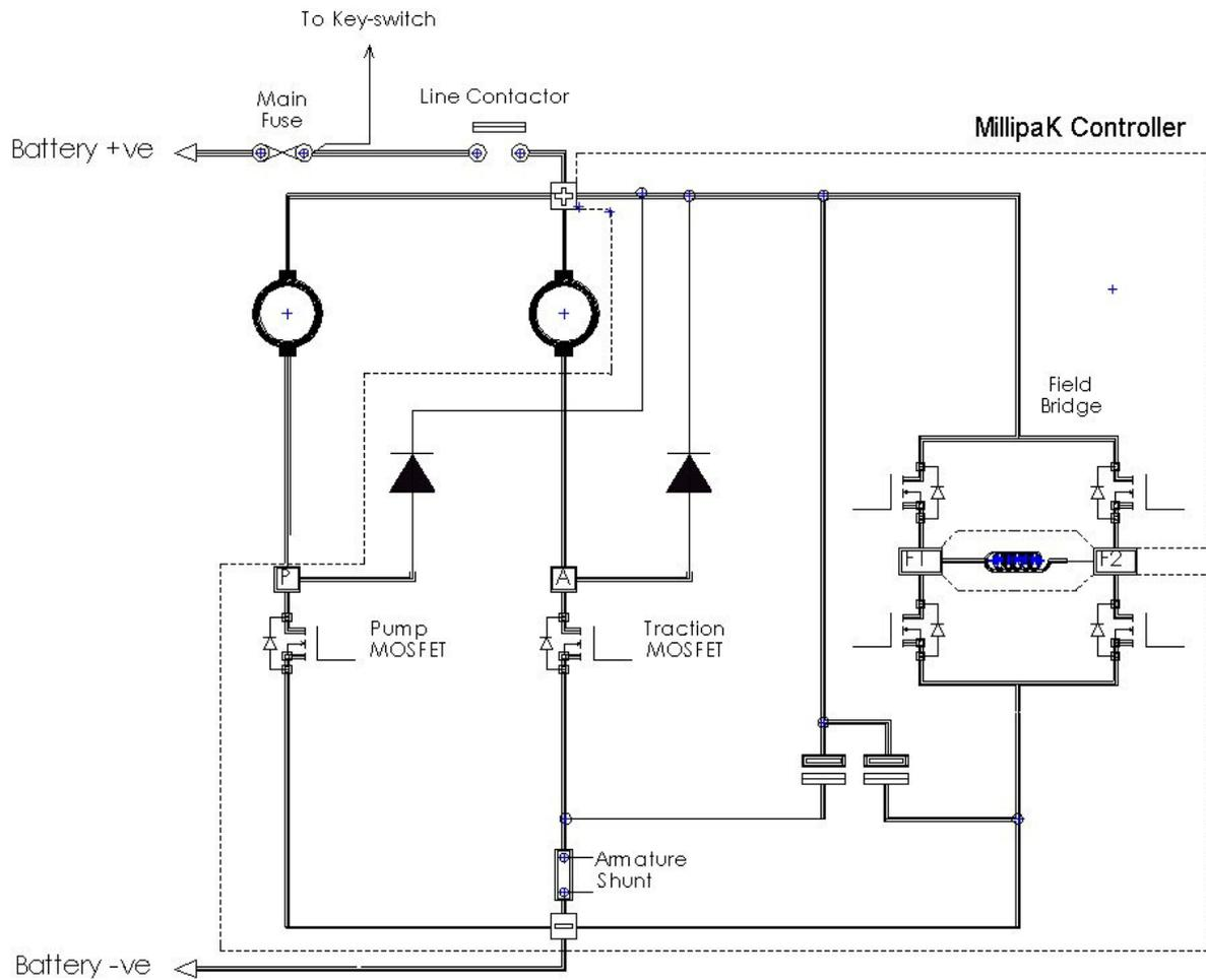
**Figure 3: MillipaK SEM Power Wiring**
