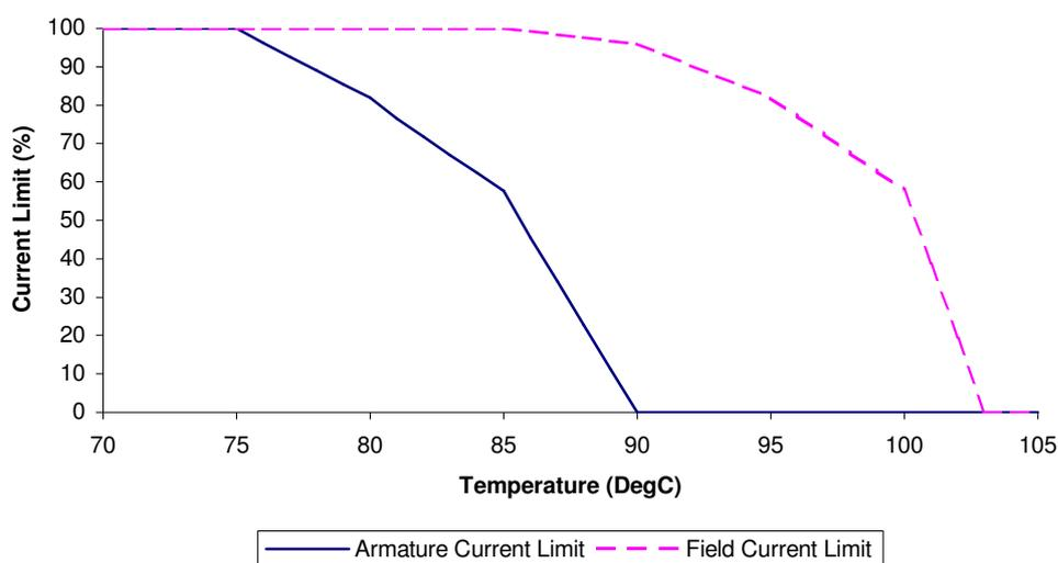
**Figure 10: Armature Thermal Cutback Characteristic**
