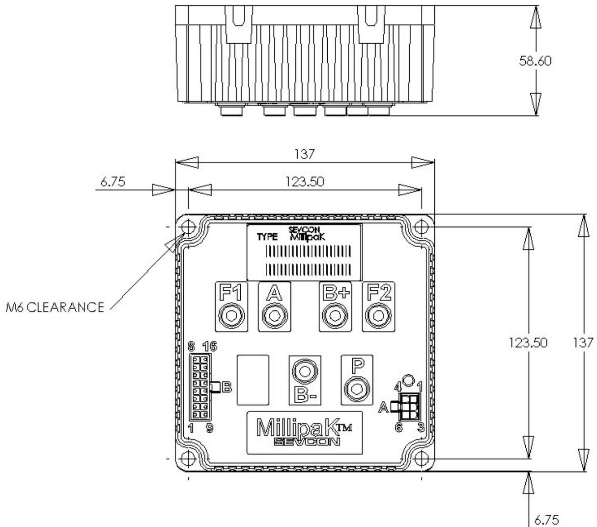
**Figure 1: MillipaK Core Dimensions**
