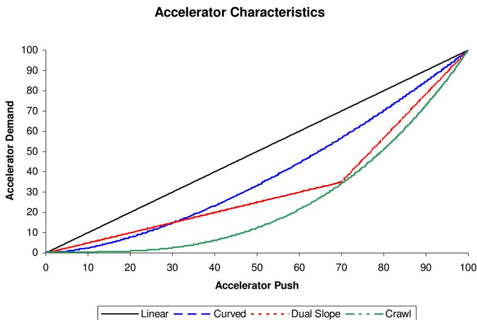
**Figure 9: Accelerator Characteristics**
