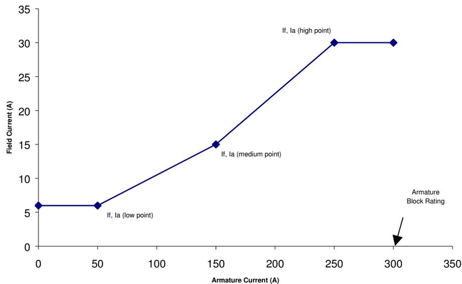
**Figure 8: Relationship between Required Field Current and Measured Armature Current**
