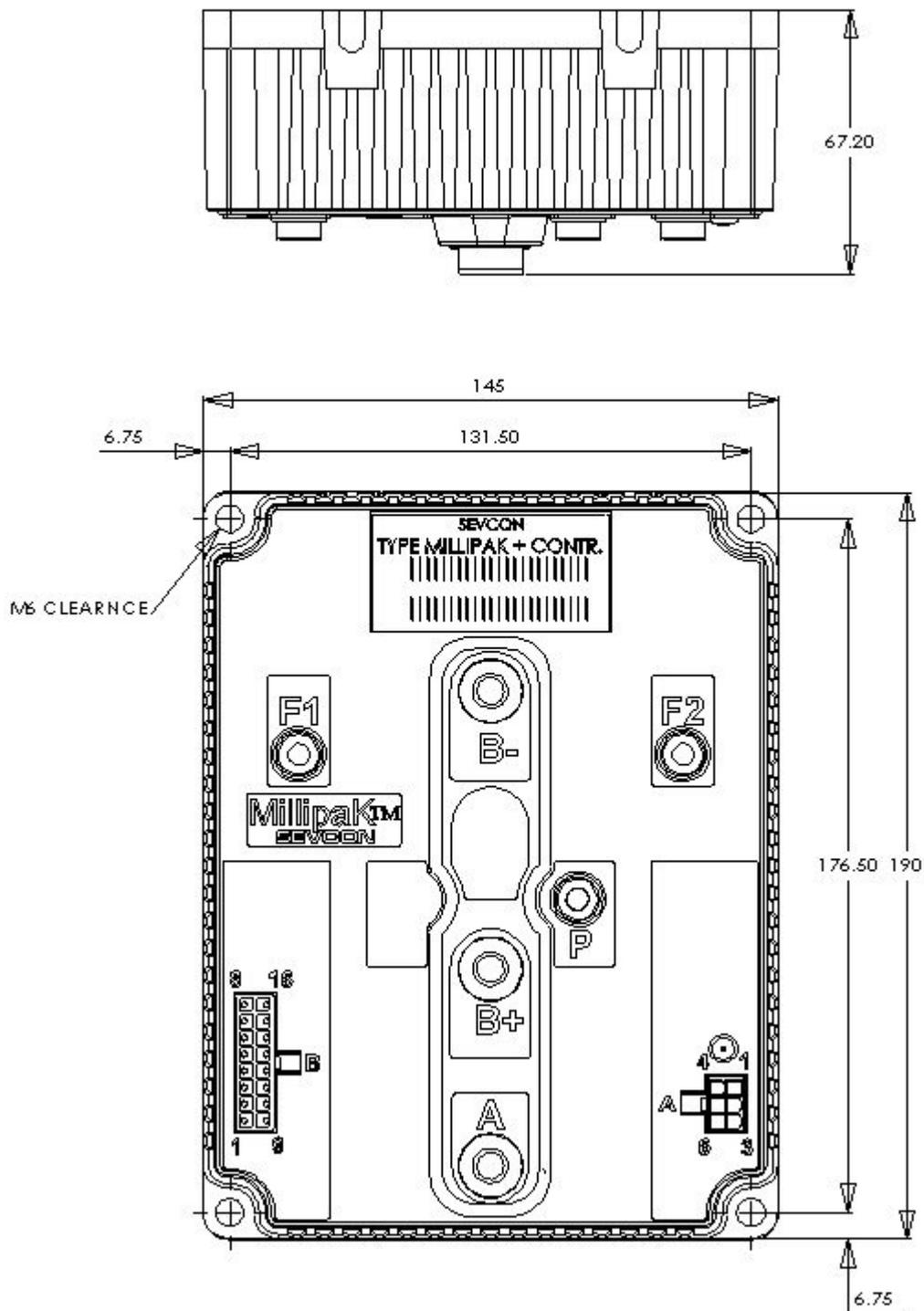
**Figure 2: Millipak HP Dimensions**
