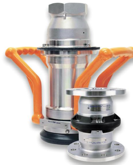
Mann Tek Safety Break Away Couplings SBC (front picture) protect hose assemblies, loading arms and pipework against excessive external loads. If the equipment is subjected to inadvertent and strong tensile loads, e.g. due to a premature movement of road and rail tankers or the drifting of ships, the coupling will separate and instantly seal the two open ends automatically.
