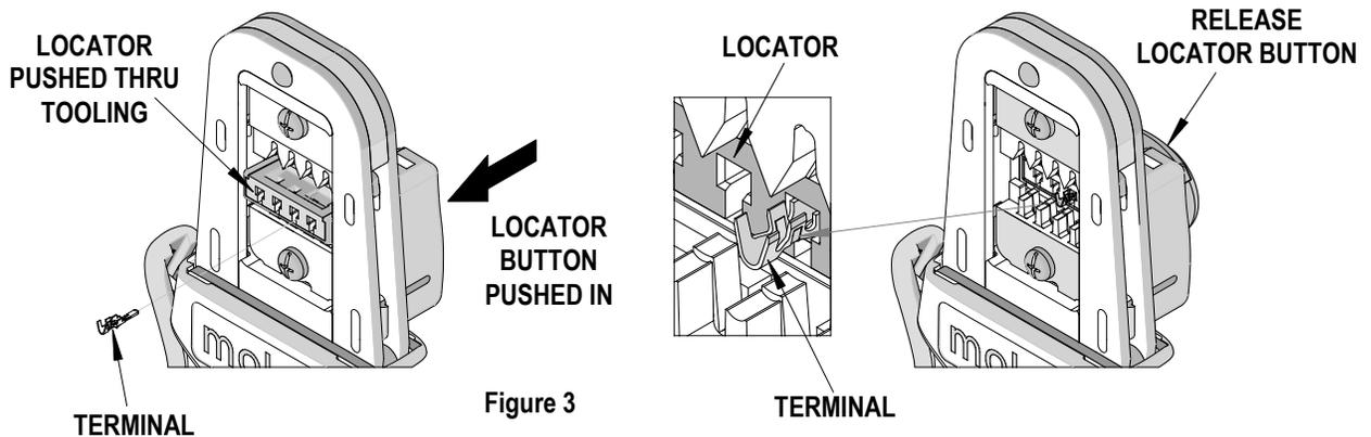
4. Release the locator button, allowing the locator to return to the crimping position.
