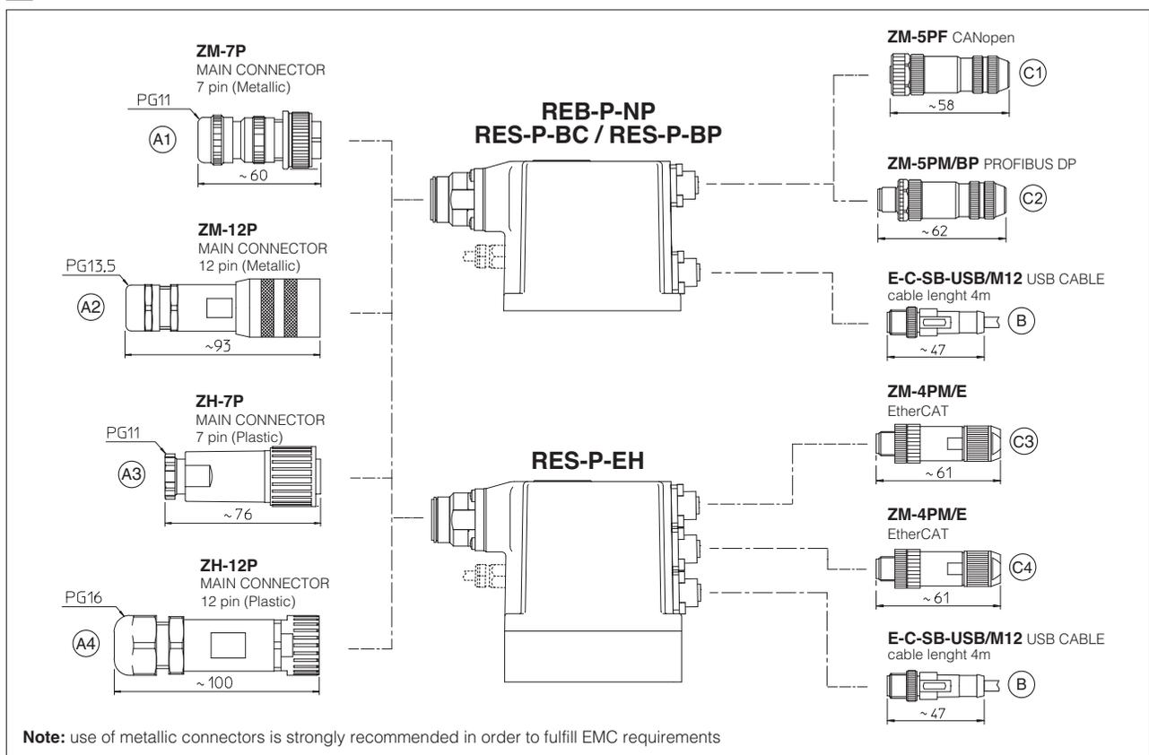
13 MODEL CODES OF MAIN CONNECTORS AND COMMUNICATION CONNECTORS - to be ordered separately
