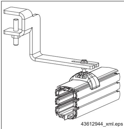
Suspension with retaining bracket on IPE or INP girder and M8 threaded pin ⇒ "Installing retaining brackets on IPE or INP girders", Page 29
