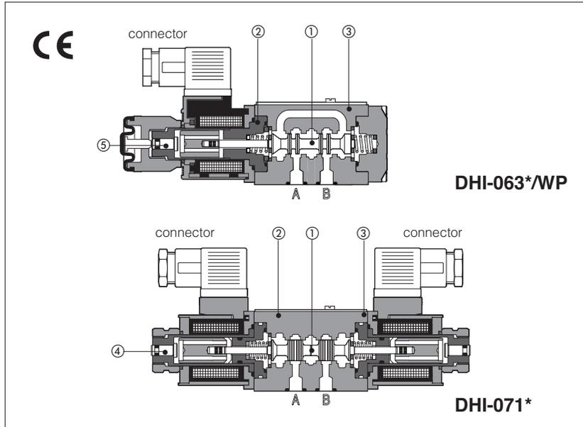
Spool type, two or three position, direct operated valves with solenoids certified according to the North American standard **cURus**.
