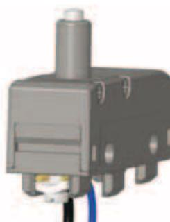
These clamping screw plates have a particular "roofing tile" structure and are connected loosely to the clamping screw. In this way, during the wires fixing, the clamping screw plate is able to suit to cables of different diameter (see picture) and tends to tighten the wires toward the screw instead of permitting them to escape towards the outside.
