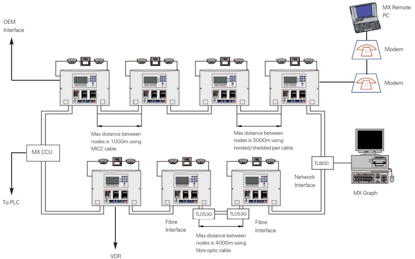
Up to 99 MX/T2000 sub-panels can be linked together providing unrivalled design flexibility (T2000 Only).
