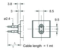
connection for AMP SUPER SEAL (two contacts) connector type code  ${\bf K8}$
