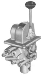
The HD-2 CONTROLAIR Valve is a composite lever operated directional valve consisting of two 3-way directional valves and a 3-way pressure regulating portion. Each unit has its own OUT port.
