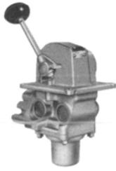
The HE-2 CONTROLAIR Valve is a composite lever operated directional valve consisting of a 3-way directional valve and a 3-way pressure regulating portion with each unit having its own OUT port.
