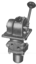
The H-2 CONTROLAIR Valve is a lever operated, 3-way, pressure regulating valve. Air pressure is increased, decreased or maintained at the OUT port according to lever position. Facing the lever side of the valve, clockwise lever movement increases pressure. (see diagram)
