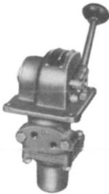
The H-2-EX and H-2-EFX CONTROLAIR Valves are 3-way pressure graduating valves which increase outlet pressures from 0 to 40% of maximum value in the first 60° of lever movement from “OFF” position, and then increases outlet pressure from 40% to maximum value in the remaining 32° of lever movement.
