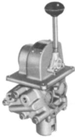
The HC-2 CONTROLAIR Valve is a lever operated, pressure regulating, 4-way directional valve. It consists of two 3-way directional valves, and a 3-way pressure regulating portion. The regulating portion furnishes the inlet air for the directional valves. Each directional valve has its own OUT port.
