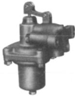
The H-3 CONTROLAIR Valve is equipped with a roller for operation by a cam or a similar mechanical device. Graduated pressure is obtained from the valve's OUT line. Total movement is approximately 5/16" (8mm) with the initial 1/16" (1.6 mm) travel used to close its exhaust valve.
