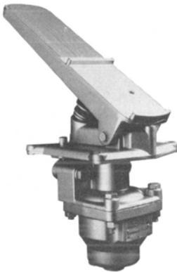
The H-1 CONTROLAIR Valve is a pedal actuated, 3-way pressure regulating valve, suitable for applications where the valve portion extends below the floor level. Depressing the pedal increases the outlet pressure. The pedal is self-returning. This valve is suitable for brake and clutch control or any use where foot operation pressure control is desired. Approx. weight: 8½ lbs. (3.9 Kg)
