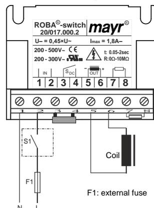
The power circuit is interrupted in front of the rectifier. The magnetic field slowly reduces. This delays the rise in braking torque.
