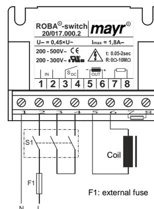
The power circuit is interrupted between the rectifier and the coil as well as mains-side. The magnetic field reduces extremely quickly. This causes a quick rise in braking torque.
