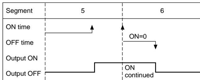
If output at the previous segment end point was ON at this time, the output status at the segment switching point does not momentarily become OFF.
