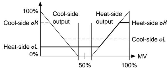
Note 3) When  $MV \geq 50\%$ , the heat-side PID set is switched to.
