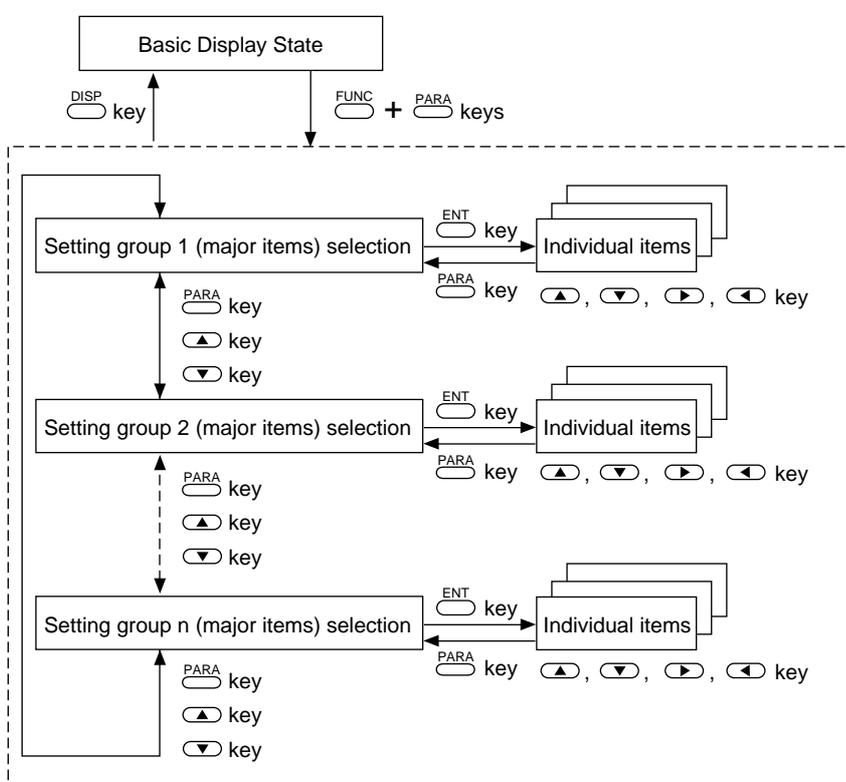
If you press  $\text{ENT}$  when the setup group to be selected is displayed, the display moves to the individual (minor) item level.
