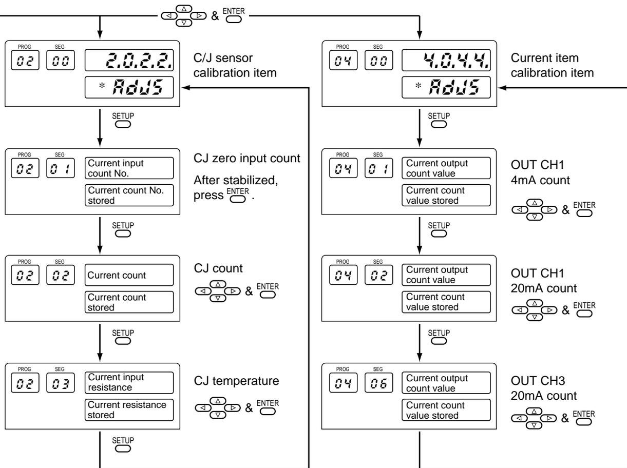
Figure 12-1. Calibration Flowchart (2/2)
