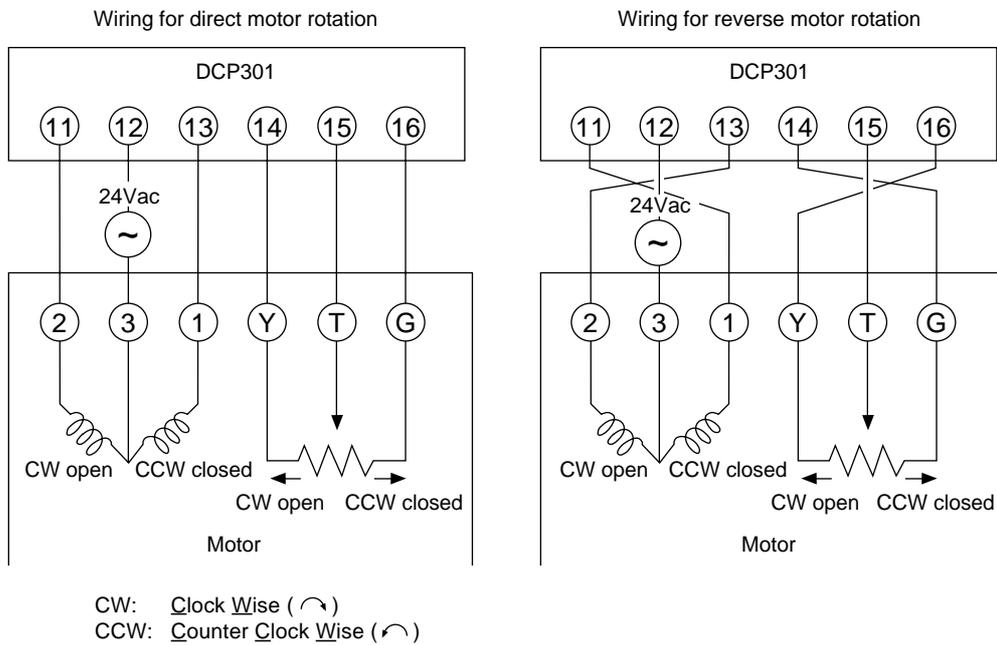
The DCP301 is also provided with a function (**AL 10** to **AL 12**) for detecting MFB disconnection or short-circuit if the motor has been wired to the controller in the wrong way.
