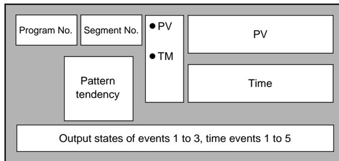
Either of “h:min” or “min:s” is selected as the time unit in setup settings. Select either “remaining segment time” or “total operating time” in setup settings as the details whose time is to be displayed.
