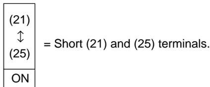
●Digital output test for control output (00-04)
