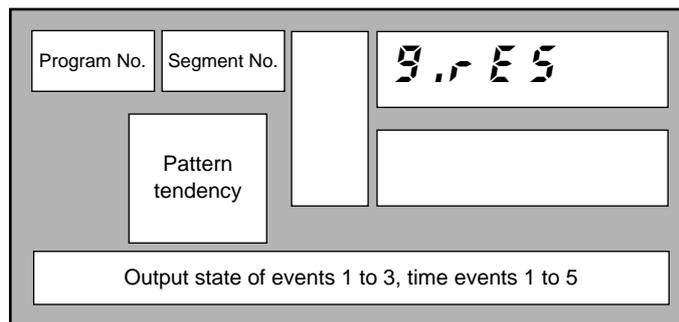
In the constant-value operation mode, all of the program No., segment No. and profiles displays are cleared.
