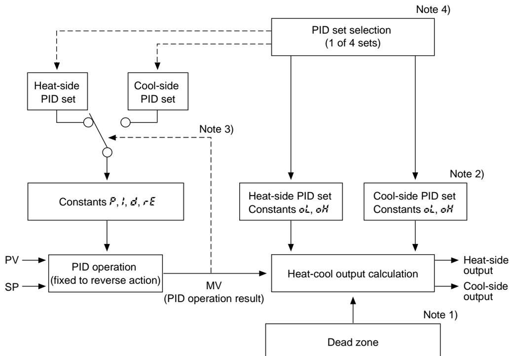
Note 1) On heat/cool models, this sets how the relationship between heat-side output and cool-side output should be processed with respect to the MV resulting from PID operation.
