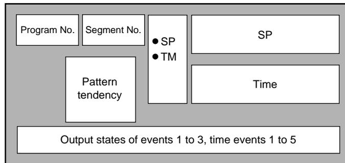
The digit to which SP values can be entered blinks in the MANUAL mode when programmer functions are selected. Either of “h:min” or “min:s” is selected as the time unit in setup settings. Select either “remaining segment time” or “total operating time” in setup settings as the details whose time is to be displayed.
