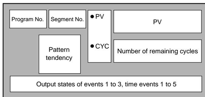
When the remaining number of cycles is “0”, subsequent cycle operation is not carried out.
