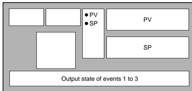
The digit to which SP values can be entered blinks in the MANUAL mode when controller functions are selected.
