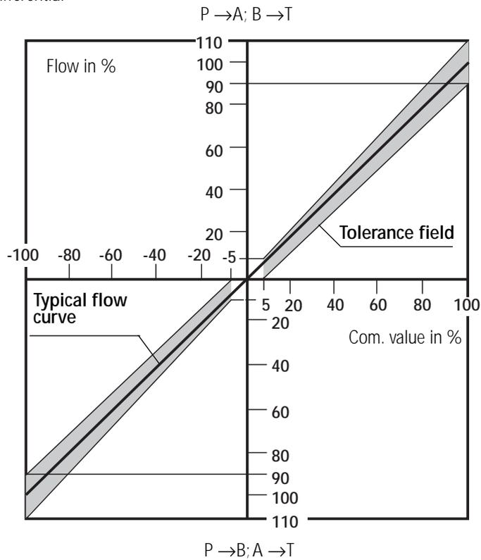
Characteristic curves (measured at  $v = 32 \text{ mm}^2/\text{s}$  and  $\vartheta = 40 \text{ }^\circ\text{C}$ )
