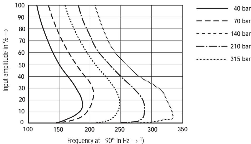
Output signal  $\hat{=}$  spool stroke with a flow without load pressure
