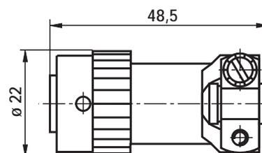
**Connection cable:** 4 or 6 core, 0,75 mm<sup>2</sup>, screened (e.g. cable type LiYCY 4 or 6 x 0.75 mm<sup>2</sup>), to DIN VDE 0812
