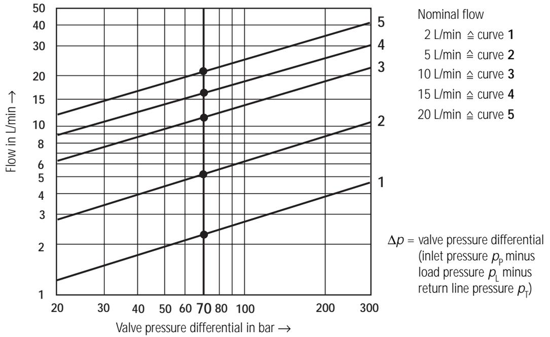
**The flow signal function tolerance field**
