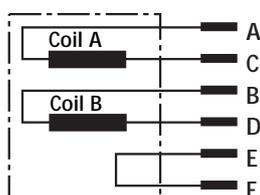
The electrical connection can either be in parallel or series. Due to reasons of operational safety and the resulting low spool inductivity, we recommend the parallel circuit.
