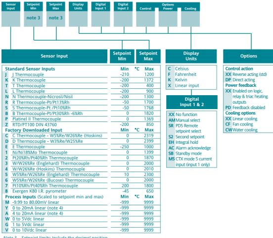
Note 3. Setpoint limits: Include the decimal position required in the displayed value. Up to one for temperature inputs, up to two for process inputs.
