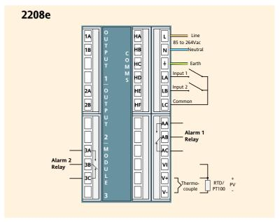
Outputs 1 and 2 are optional outputs which can be any one of the types shown in the tables below. They can be configured for heating, cooling or alarms.
