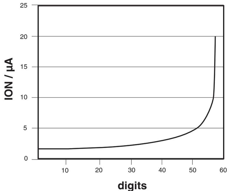
The quality of the flame signal is displayed for flame guard 1 as a number between 0 and 58.
