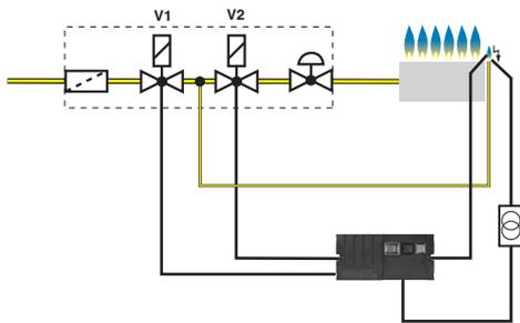
Atmospheric burner with ignition gas output.
