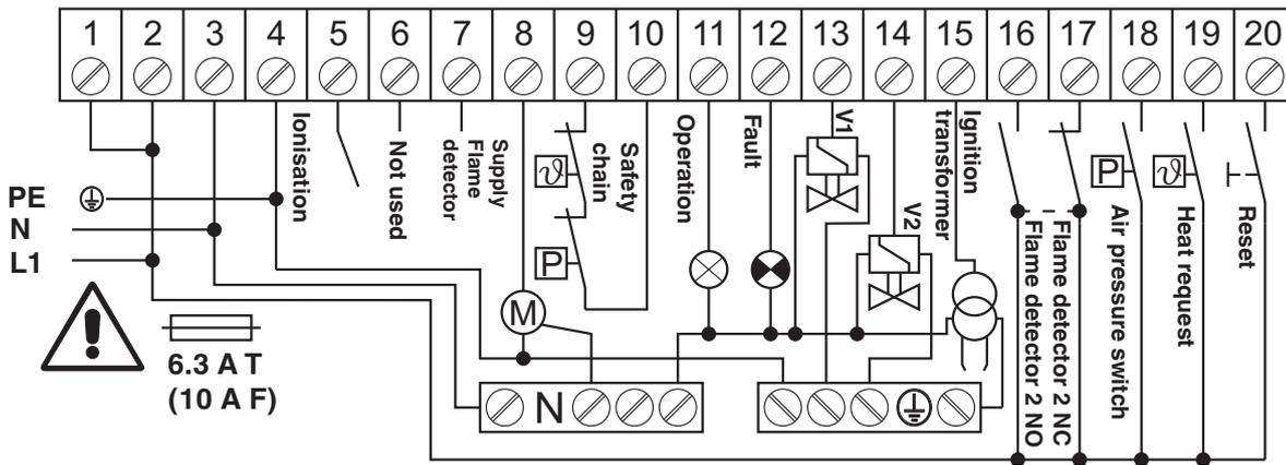
The wires which are used for the connection must be approved for ambient temperatures of minimum 75 °C (167 °F).
