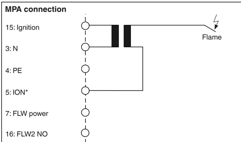
\*When using a DUNGS DEZ 1xx SEO ignition transformer for single-electrode operation, the green/yellow cable must be connected to terminal 5.
