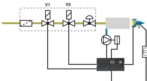
Fan burner, direct ignition of the main gas flame.
