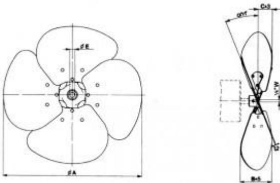
Cote d'encombrement : A = 400mm, B = 125mm, C = 60mm, E = 12,7mm
