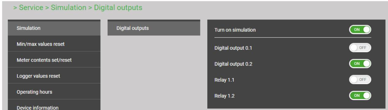
Simulation of digital outputs via device webpage
