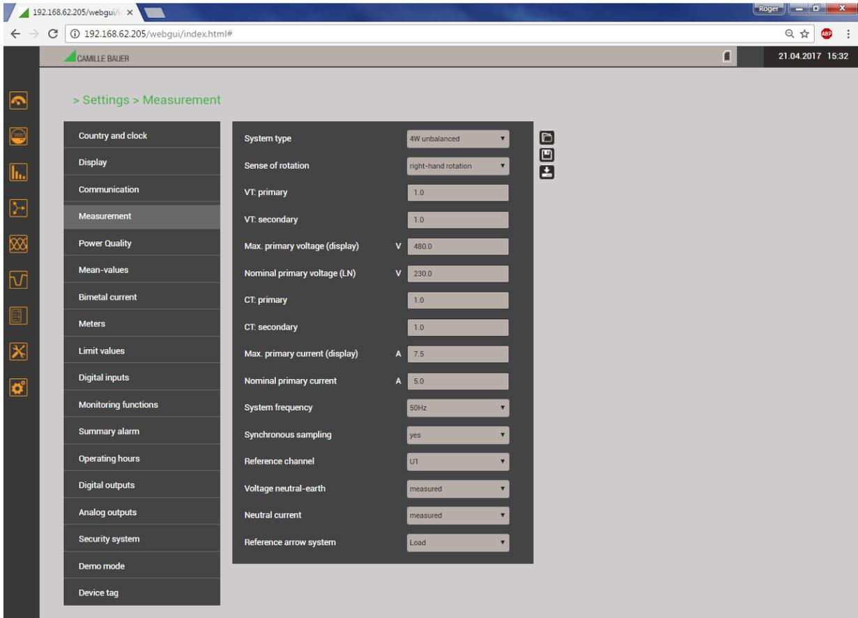
Via WEB-GUI all device settings can be performed as via the local GUI. Possibly modifications needs to be saved in the device, before all parameters have been set. In such a case the following message appears:
