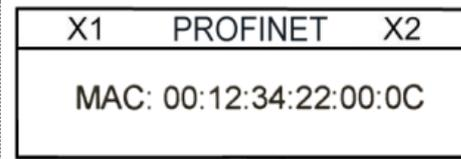
Typically, for a PROFINET device [3 MAC addresses](#) are required:
