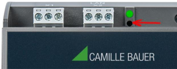
If the communication settings of the Standard interface are no longer known, they can be reset to the default settings by pressing the sunk-in reset button (located below the operating LED) for at least 3s. During the reset the operating LED flashes red. After the reset the device is rebooted.
