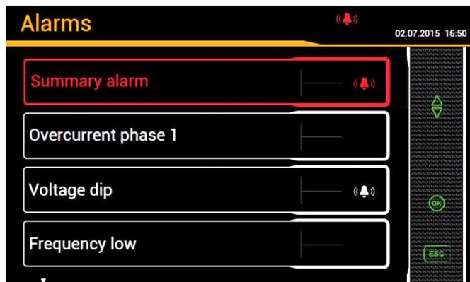
The digital or relay output assigned to the summary alarm can be reset by means of the <OK> key. So the active alarming will be stopped. But the alarm state of the summary alarm remains active until the alarm state no longer exists.
