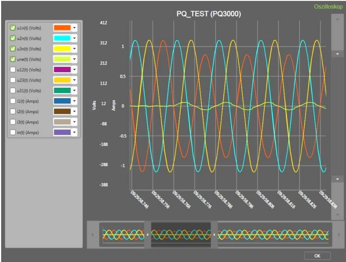
*Representation of a voltage dip, using the SmartCollect PM20 software*
