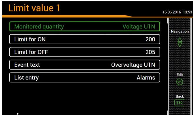
Using limit values either the exceeding of a given value (upper limit) or the fall below a given value (lower limit) is monitored.
