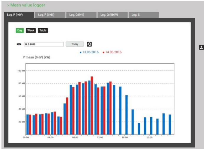
The selection of the mean-value quantity to display can be performed via choosing the corresponding register. Three different kind of displays are supported:
