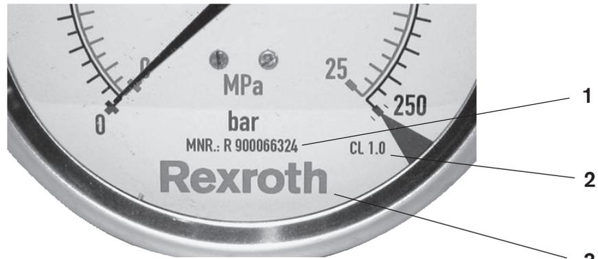
On dual scales, the lettering of the outer scale division (bar) is black, that of the inner scale division red.
