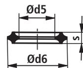
Seal ring for metal sealing. After sealing has been achieved, the pressure gauge can still be turned by 360°, so that any desired position can be set.
