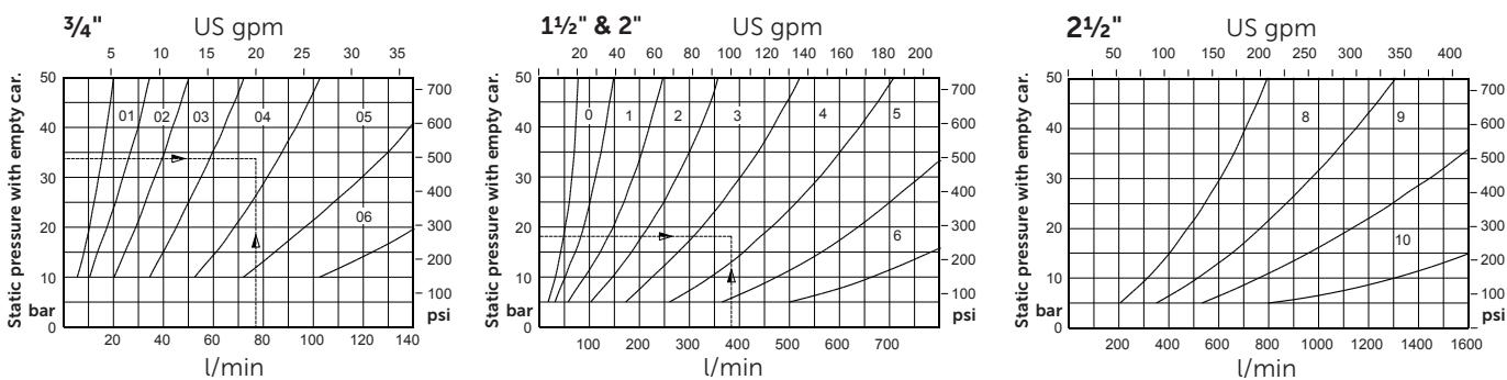
To order EV: Size (inch), valve type, state pump flow, empty car pressure (or flow guide size) and solenoid voltage.
