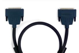
**SH6868**—Shielded 68-pin cable terminated with two 68-pin 0.050 series D-type connectors. Cable is used to connect NI 4350 and NI 4351 devices to 68-pin accessories.
