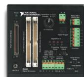
**PCB Mounting Connectors for Custom Accessories**—Build custom accessories that connect to 68-conductor shielded and ribbon cables using these connectors.
