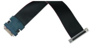
**R6868**—A low-cost, 68-conductor flat ribbon cable terminated with two 68-pin connectors. Use this cable to connect a 68-pin E Series, S Series (except NI 6143), or B Series multifunction DAQ device to 68-pin accessories.
