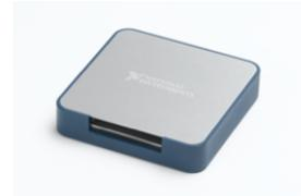
**SCB-68**—Shielded I/O connector block for rugged, low-noise signal termination with 68-pin DAQ devices. It includes general-purpose breadboard areas and an IC temperature sensor for cold-junction compensation in temperature measurements.
