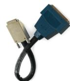
**SHC68-NT-S**—A shielded 68-conductor cable terminated with a 68-pin male VHDCI connector at one end and open to bare wires at the other. The cable connects M Series, NI 6143, and R Series devices to custom accessories through bare wires.
