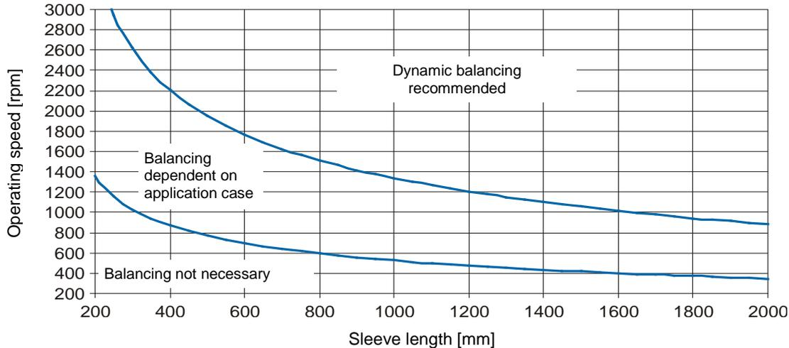
Smooth running of the machine is not only ensured by the coupling balance quality, but is also influenced by parameters such as rigidity and distance to the adjacent bearings as well as by the sensitivity and mass of the entire construction.
