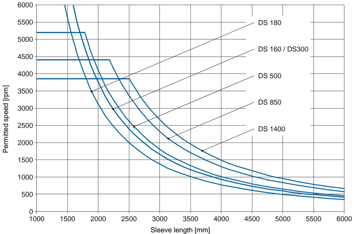
**Diagram 4: Permitted Speeds (Bend-critical) for Sleeves CFRP Type 951.\_ \_5**
