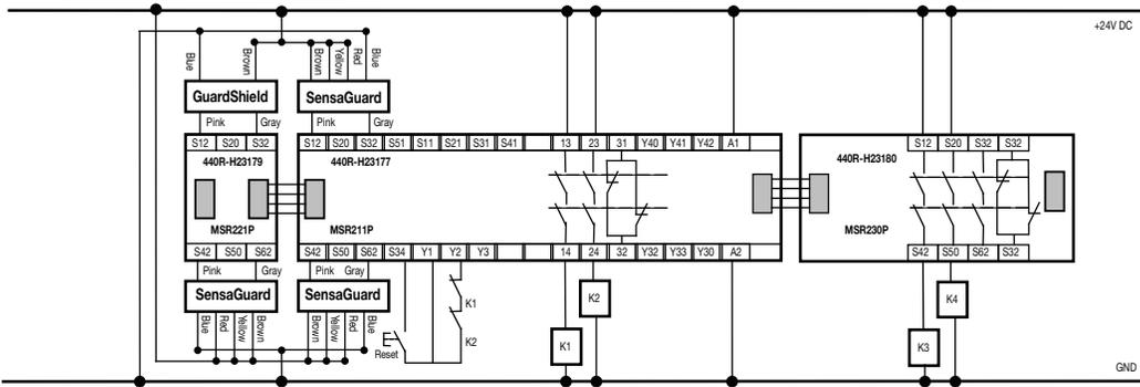
MSR200 series with 3 sensors and 1 440L light curtain, manual reset, driving 100S or 700S safety contactors.
