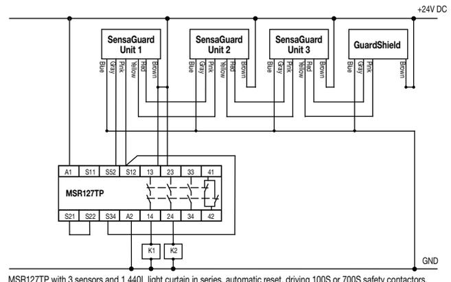
MSR127TP with 3 sensors and 1 440L light curtain in series, automatic reset, driving 100S or 700S safety contactors.
