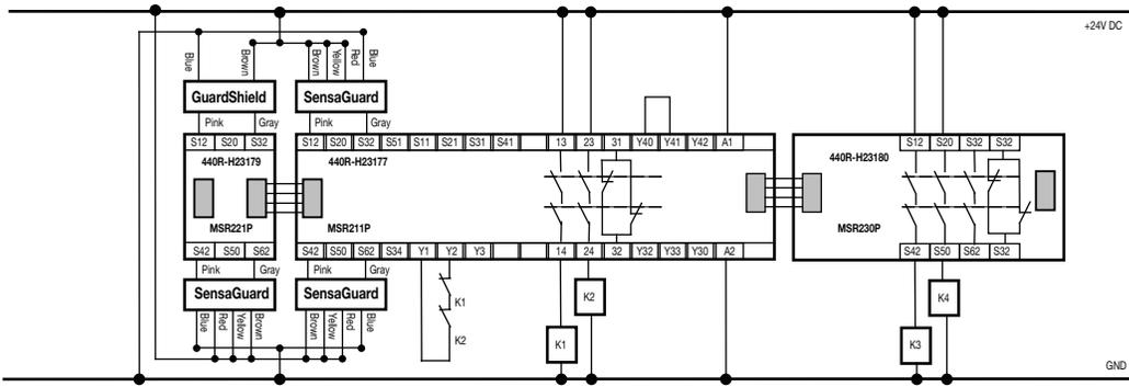
MSR200 series with 3 sensors and 1 440L light curtain, automatic reset, driving 100S or 700S safety contactors.
