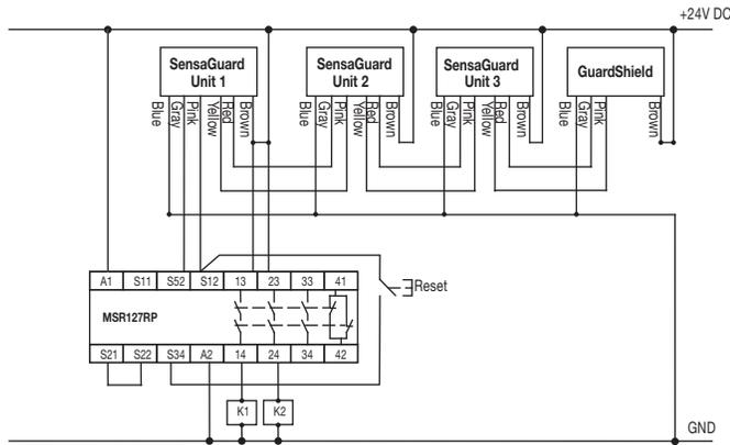
MSR127RP with 3 sensors and 1 440L light curtain in series, monitored manual reset, driving 100S or 700S safety relays.
