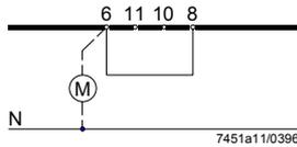
If the case of burners with no air damper (or with an air damper not controlled and monitored by the burner control), terminals 8 and 6 must be linked, as otherwise the burner control will not be able to start the burner.
