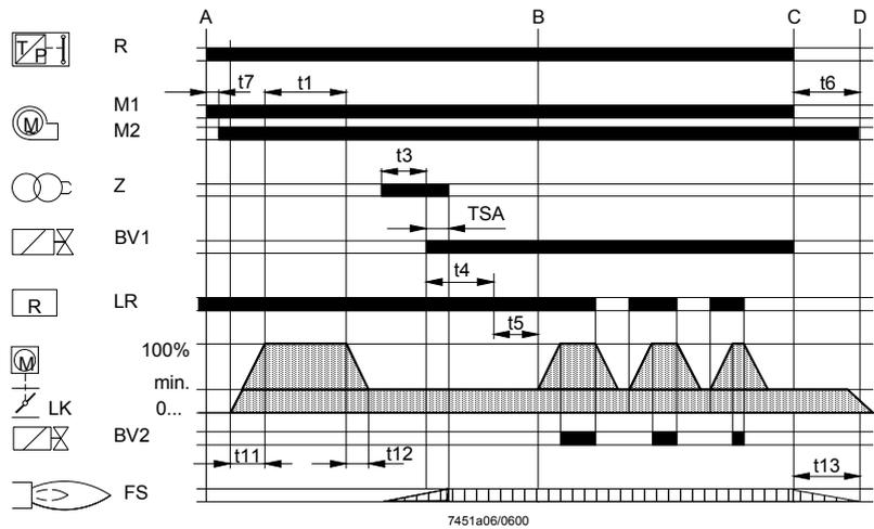
Control of actuator «SA» according to the single-wire principle (actuator «SA»: E.g. SQN3... as per Data Sheet 7808). For other connections, refer to «Connection diagrams».
