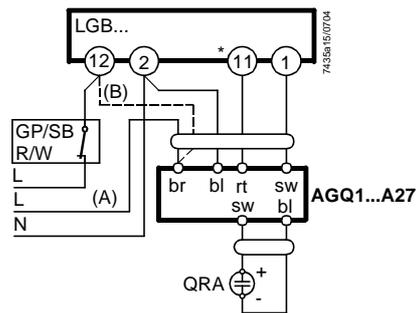
Measurement made on the flame detector
