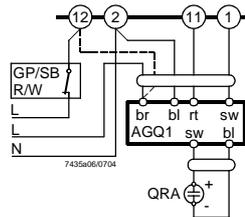
Burner with fan control via auxiliary contactor («HS») **with «LP»**
