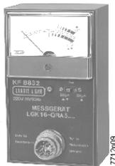
**KF8832** unit for measuring the detector current
