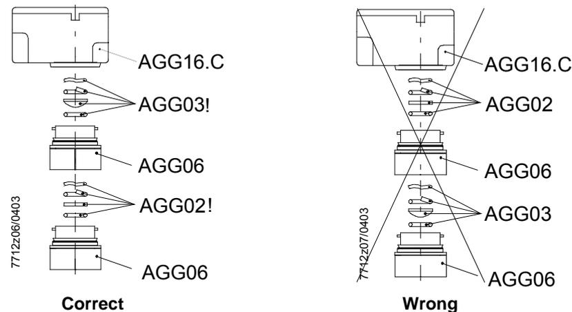
AGG06 has a bayonet fitting with which it is attached either to the housing of the AGG16.C or to the housing of the QRA10... and the 1 in. mounting coupling.
