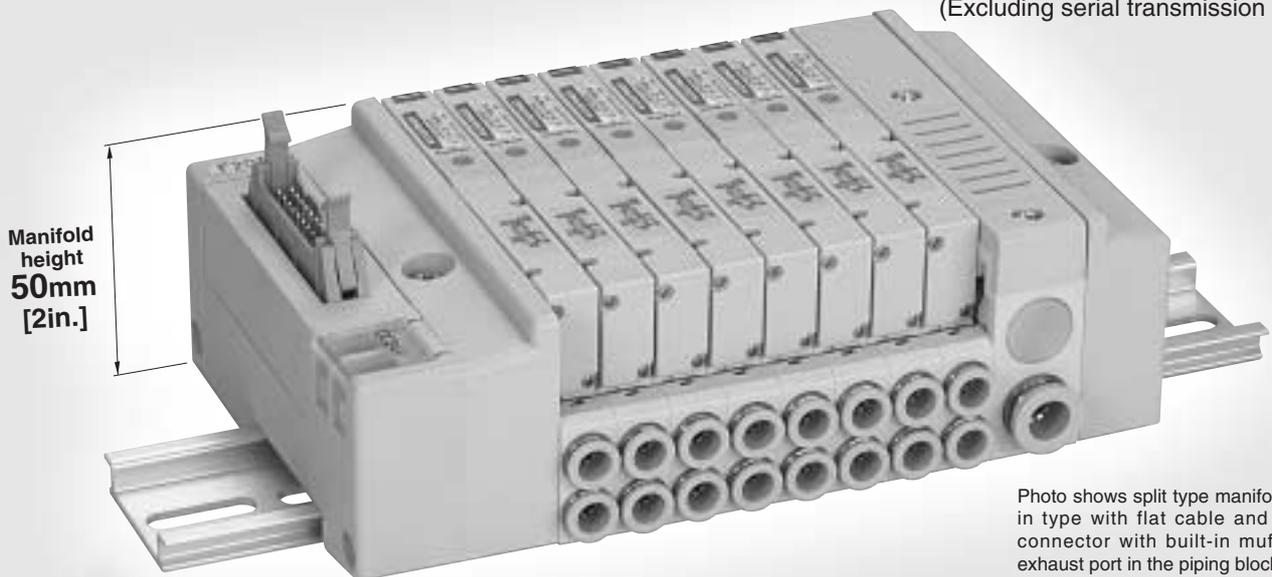
Photo shows split type manifold plug-in type with flat cable and 20-pin connector with built-in muffler on exhaust port in the piping block.
