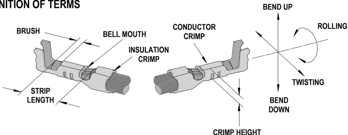
The above terminal drawing is a generic terminal representation. It is not an image of a terminal listed in the scope.
