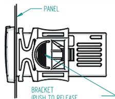
Instrument **XR77CX** shall be mounted on vertical panel, in a 29x71 mm hole, and fixed using the special bracket supplied. The temperature range allowed for correct operation is 0 to 60°C. Avoid places subject to strong vibrations, corrosive gases, excessive dirt or humidity. The same recommendations apply to probes. Let air circulate by the cooling holes.
