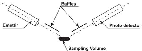
Fig. 1 System schematic
