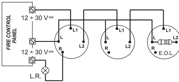
Fig. 2 Connection diagram.
