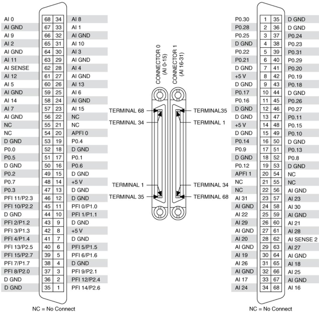
NI PCI/PXI-6254 Pinout
