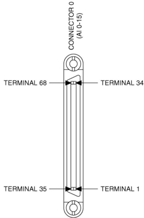
NI PCI/PXI-6250 Pinout
