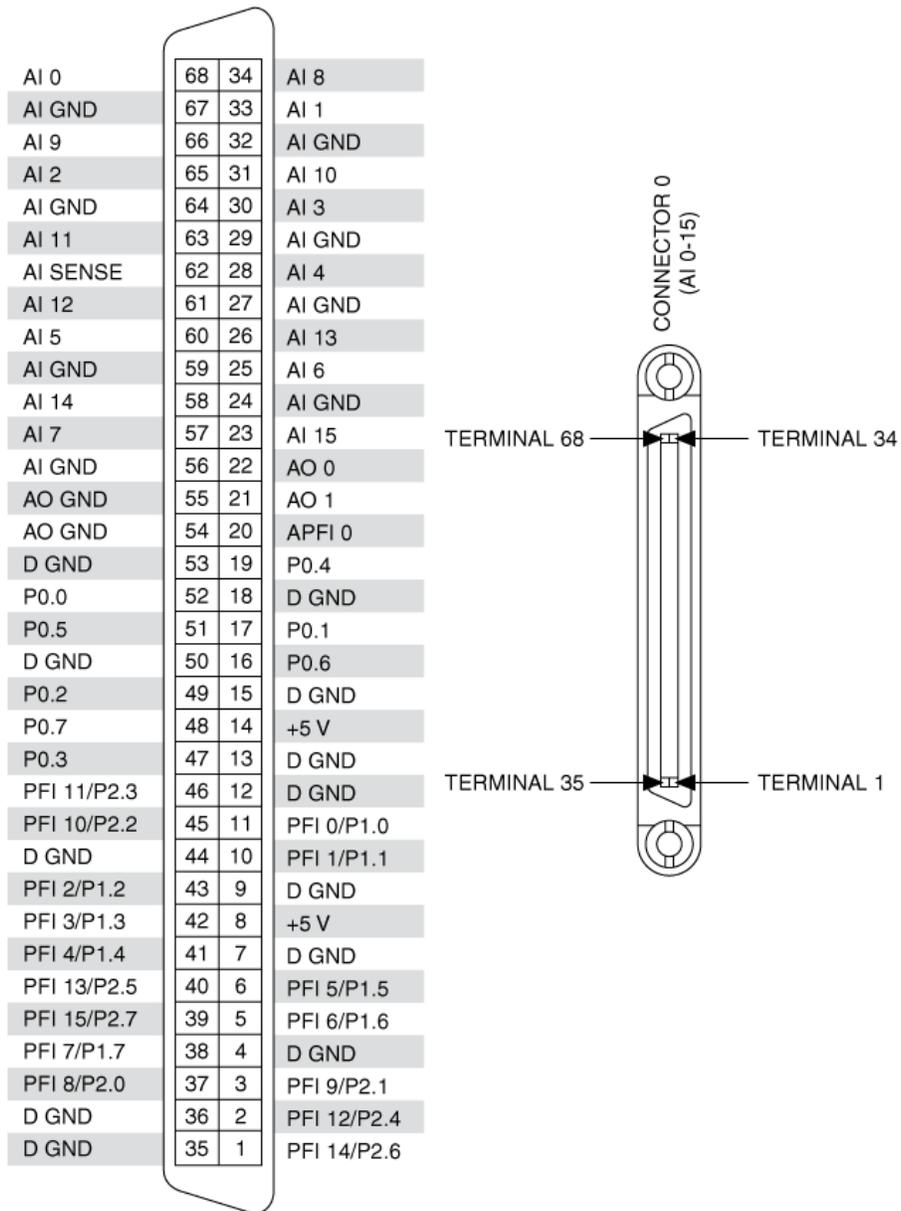
NI PCI/PCIe/PXI/PXIe-6251 Pinout
