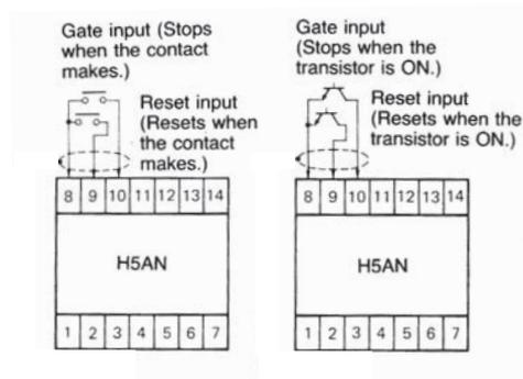
When connecting a transistor circuit not of the open collector type to the gate or reset inputs as shown below, the voltage of the transistor circuit (+V) should be 13 to 30 V, and the  $V_{CE(S)}$  of the transistor should be less than 3 V (the current that flows from either terminal 9 or 10 is approximately 10 mA). Moreover, it is essential that the circuit be ON for gate or reset input, and OFF when there is no input.
