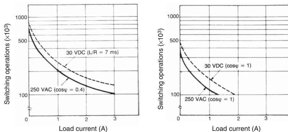
Reference: A maximum current of 0.15 A can be switched at 125 VDC (cosφ = 1).
