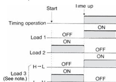
Note: Output transistor ON: Low (0 V)
