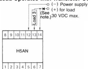
Note: Connect a diode when using a Power Supply of 12 V or less.
