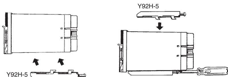
Turn the screws on the mounting brackets counterclockwise to loosen them sufficiently. Attach the bottom mounting bracket first.
