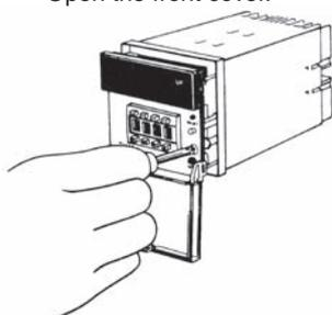
The internal unit comes out by loosening the internal unit fixing screw.
