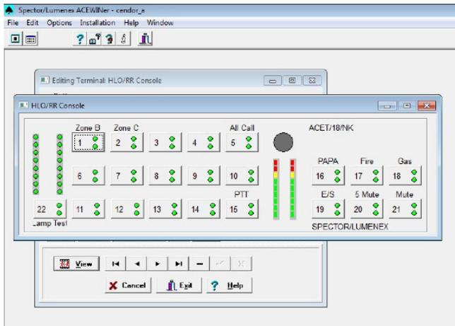
Where there is more than one ACE100 node then this Window allows the engineer to declare which node port a source input is connected to.
